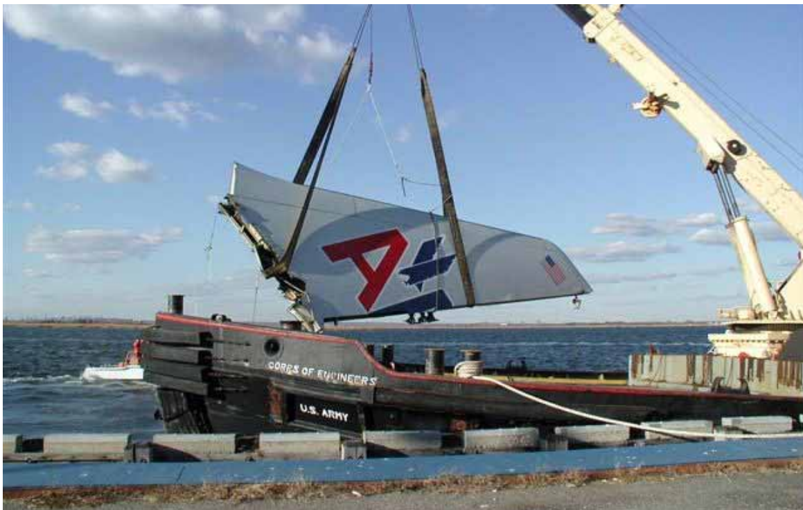
Figure 11. Vertical Stabilizer After Recovery From Jamaica Bay
