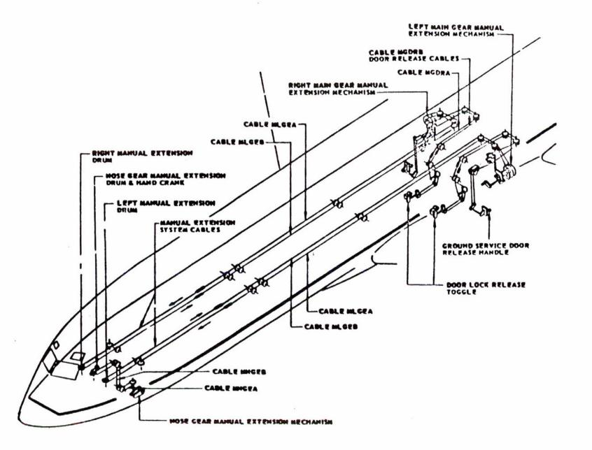
Figure 1.-Manual gear extension system.
