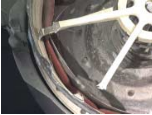
Figure 234: Outer diaphragm, intact (not torn) portion.
