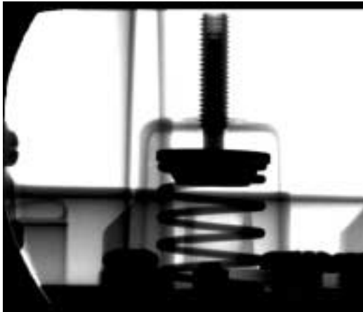
Figure 259: Integral control adjustment spring.
