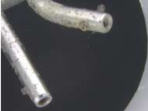
Figure 110: Aft hinge pins, upper & lower. Aft/lower pin is rotated to non-closed door position.
