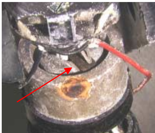
Figure 17: LEFT, OUTFLOW VALVES Position Indicator witness mark
