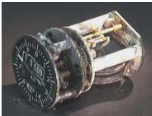
Figure 44: Cabin Altitude Indicator, housing removed.
