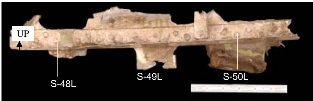
Figure 1.16-105 As received condition of the STA 2160 frame segment submitted for examination. The aft surface is shown in this view.
