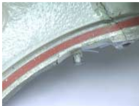
Figure 194: Exterior door open, stop pin, HS P/N 730539-1. Overview of forward/upper pin as viewed from inside. • Appears to be normal and not bent relative to valve housing.
