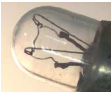
Figure 38: PRESS RELIEF light, upper, left lamp, (filament intact) - (Ref. Figure 37, yellow arrow for lamp location).
