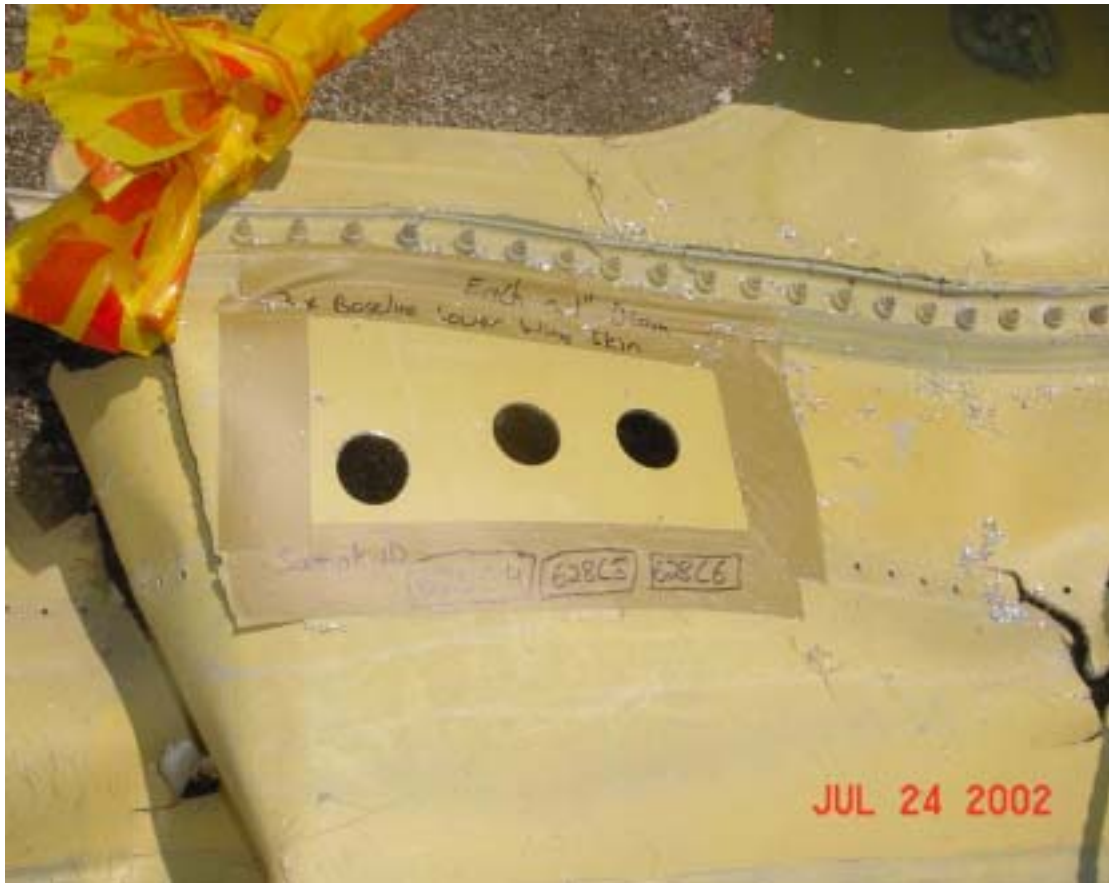
Figure 1.16-167 Discoloration sample 628, showing the locations of samples 628C4, 628C5 and 628C6.
