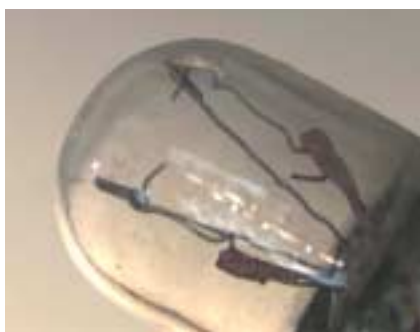
Figure 40: PRESS RELIEF light, lower left lamp. • Filament is broken - (Ref. Figure 37, red arrow for lamp location).
