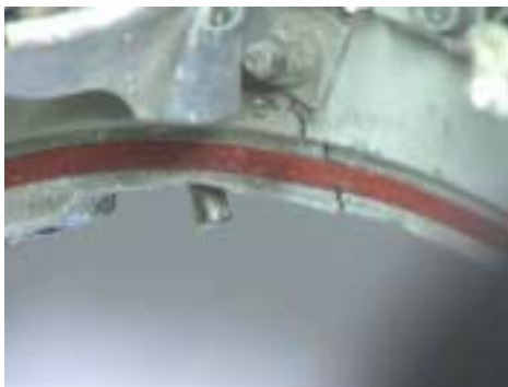
Figure 204: Exterior door open, forward/lower stop pin, HS P/N 730539-1, as viewed from inside.
