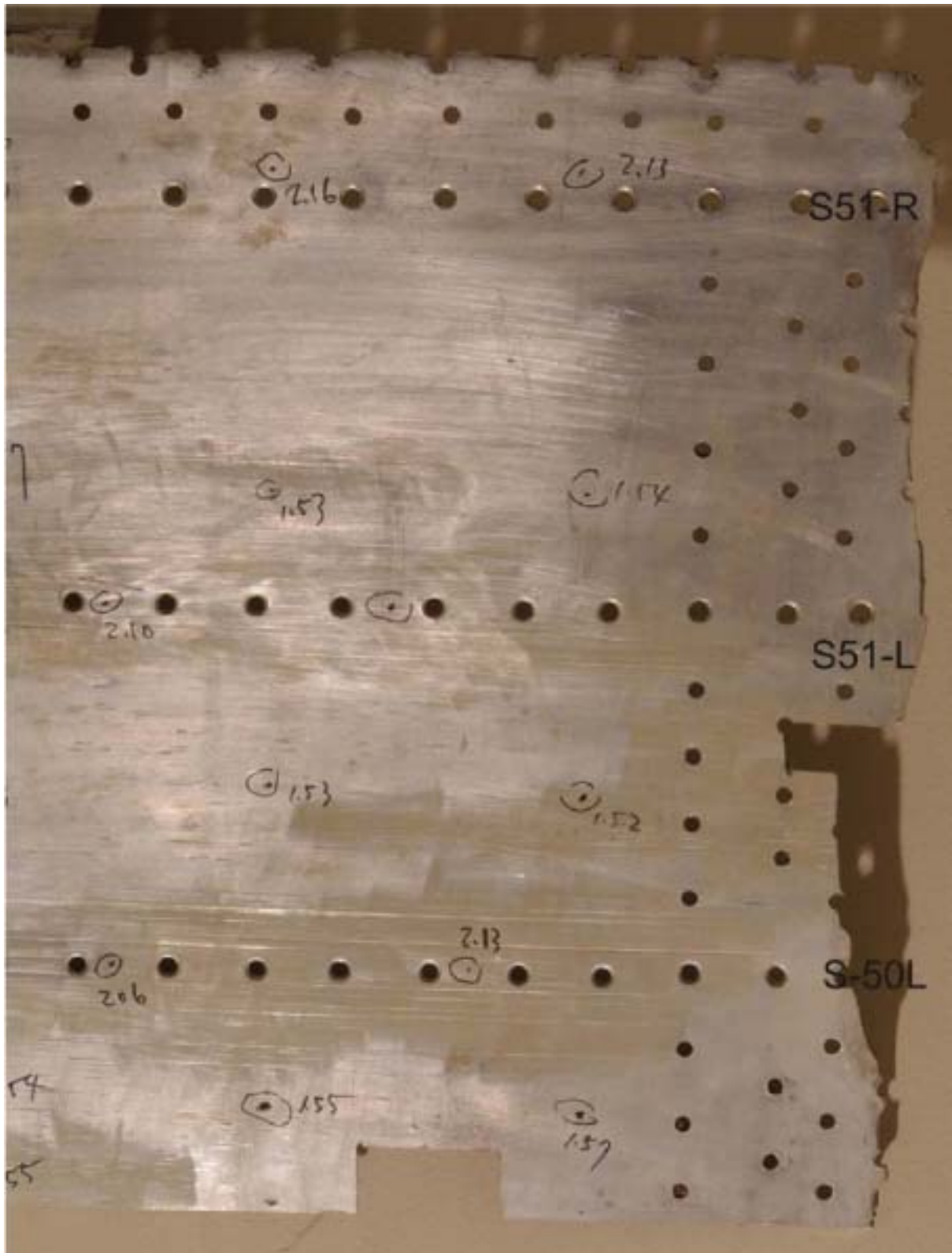
Figure 1.16-70 Extent of damage consistent with a tail strike
