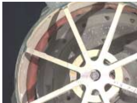
Figure 147: Diaphragm, apparently intact portion.
