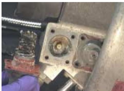
Figure 250: Showing remote ambient sensor removed.
