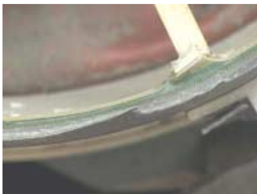
Figure 140: Close-up of knife-edge damage.
