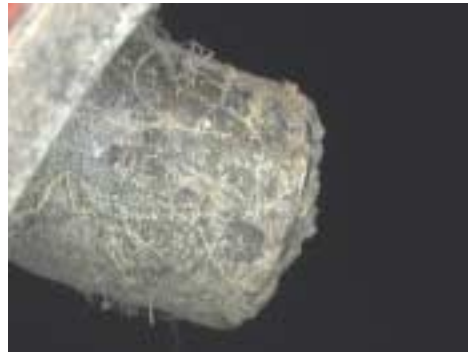
Figure 123 : Aft/upper stop pin; close up of figure #122.
