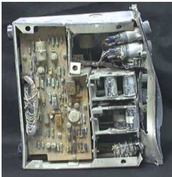
Figure 9: Flight Engineer's Cabin Pressure Control Selector Panel - (top view)
