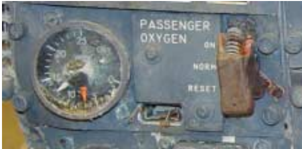
Figure 53: Passenger Oxygen Panel, module M183.
