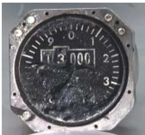
Figure 43: Cabin Altimeter Indicator, glass bezel removed
