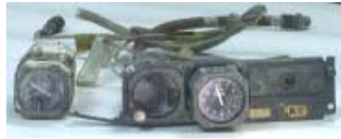
Figure 3 : Flight Engineer's Cabin Altitude Pressure Module
