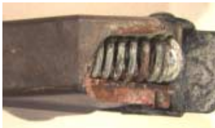
Figure 61 : Top view of switch guard damage.
