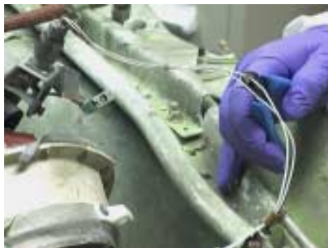
Figure 180: Lower Pressure Relief Valve. Cut switch lead wire A, step 1 in removal of lower valve (before cut).
