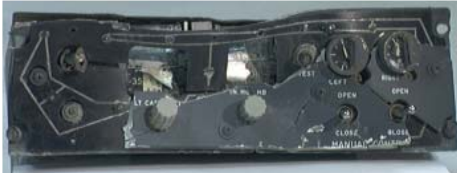
Figure 1.16-1 Flight Engineer's Cabin Pressure Control Selector Panel
