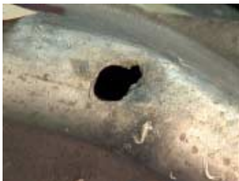
Figure 209: Hole penetrating support housing, HS P/N 727405-1.
