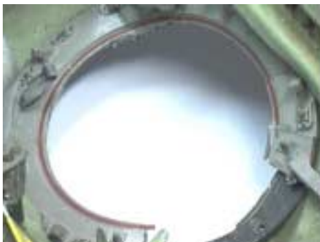
Figure 193: Non-metallic washer (gate seal), HS P/N 527355-13, as viewed from inside. • Approximately 25% of seal is missing. • Slight impression of gate knife-edge on seal surface. • No abnormal cuts on seal surface.
