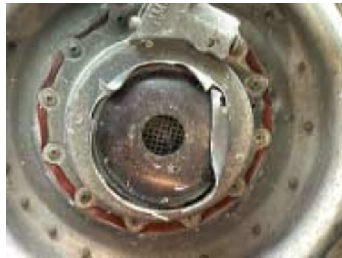
Figure 239: Overall of control, filter end. • Filter cover HS P/N 727423-1 & spring HS P/N 727430-1 are missing. • Filter housing HS P/N 727426-1 is bent over holding filter in place.
