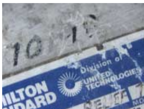
Figure 174: Lower Pressure Relief Valve data plate, identified FT 10/98 with microscope.
