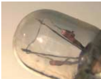
Figure 38: PRESS RELIEF light, upper, left lamp, (filament intact) - (Ref. Figure 37, yellow arrow for lamp location).
