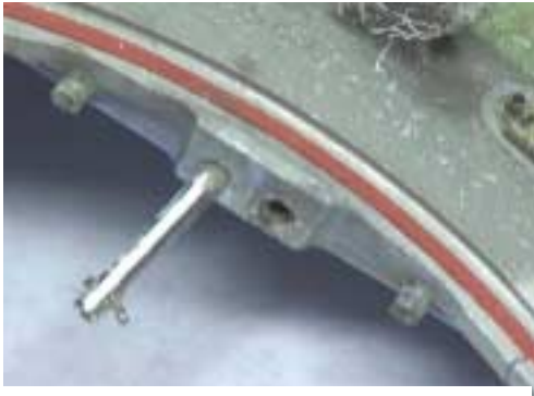
Figure 101: Forward stops & hinge pin, (looking from inside to outside). • Forward/lower hinge pin is missing.
