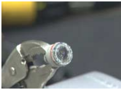
Figure 257: Plug for integral sensor, seal looks normal and uncut.
