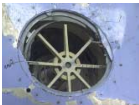
Figure 83: Upper Pressure Relief Valve, orientation as installed on airplane.
