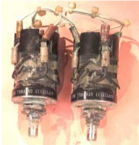
Figure 31: BLEED AIR switches #1 & #2 overview
