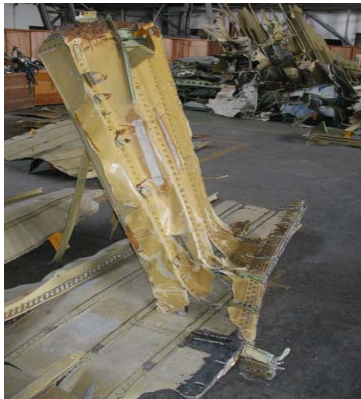
Figure 1.12-10 The recovered and identified portions of the Wing Center Section front spar
