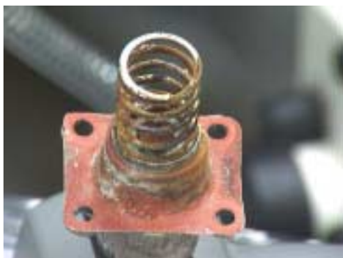
Figure 171: Integral ambient sensor spring & diaphragm.
