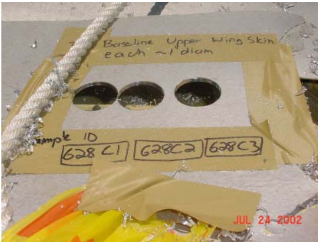
Figure 1.16-166 Discoloration sample, showing the locations of samples 628C1, 628C2 and 628C3.
