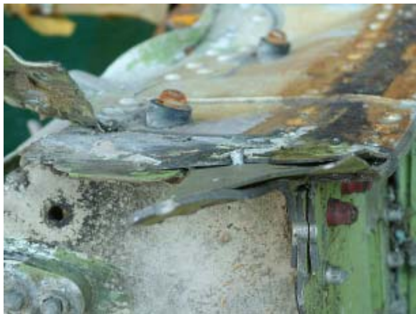
Figure 1.16-155 Macro examination of the fractography down below the patch.(0.53X)
