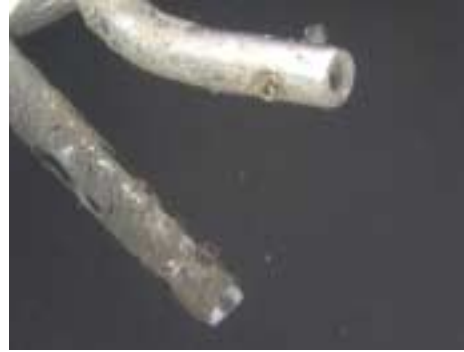
Figure 111: Aft hinge pins, upper & lower. Both pins rotated to "closed door" position.
