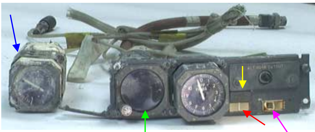
Figure 37: M188 panel. Note that the vertical speed indicator was detached from the module.
