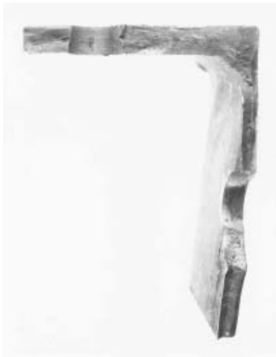
Figure 1.16-153 Macro examination of Left fractography as in figure 2.(2.3X)
