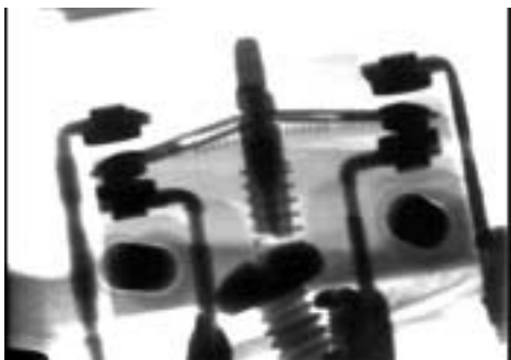
Figure 248: Lower Pressure Relief Valve, closed valve switch; "Not Closed" contacts.
