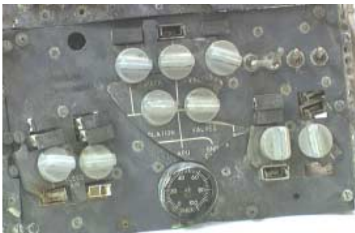
Figure 23: Detail overview of the M170 portion of the Flight Engineer's Panel.
