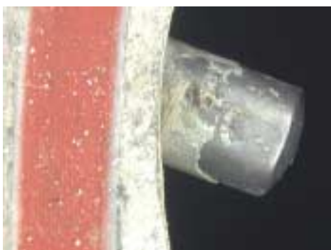
Figure 193: Non-metallic washer (gate seal), HS P/N 527355-13, as viewed from inside. • Approximately 25% of seal is missing. • Slight impression of gate knife-edge on seal surface. • No abnormal cuts on seal surface.
