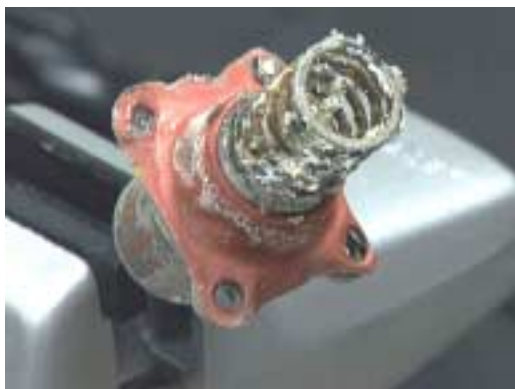
Figure 255: Integral sensor spring and diaphragm.
