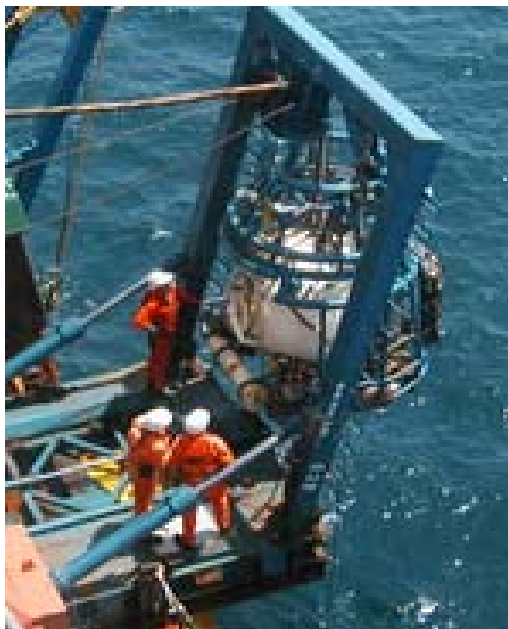
Figure 1.18-9 (a) The salvage vessel Jan Steen- upper-right photo, (b) a saturation diving chamber - left photo, (c) a 100 HP ROV on Jan Steen- lower-right photo
