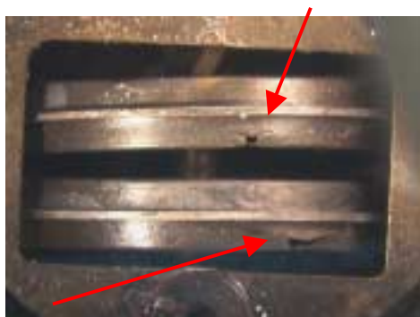
Figure 46: Cabin Altimeter Indicator, bellows, visible damage
