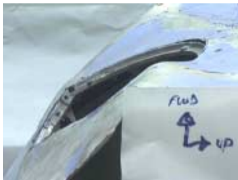
Figure 183 : Skin distortion at valve mounting location.
