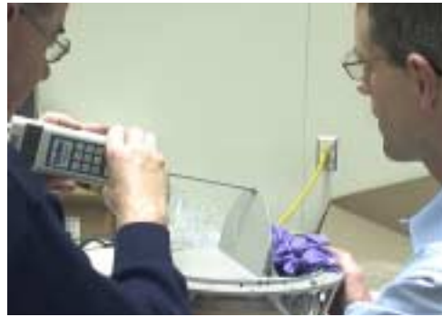
Figure 270: Comparison unit*, door B compression (closing), 1.95 pounds (push at center of door to close door).
