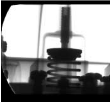
Figure 244: Integral sense control, adjustment spring.
