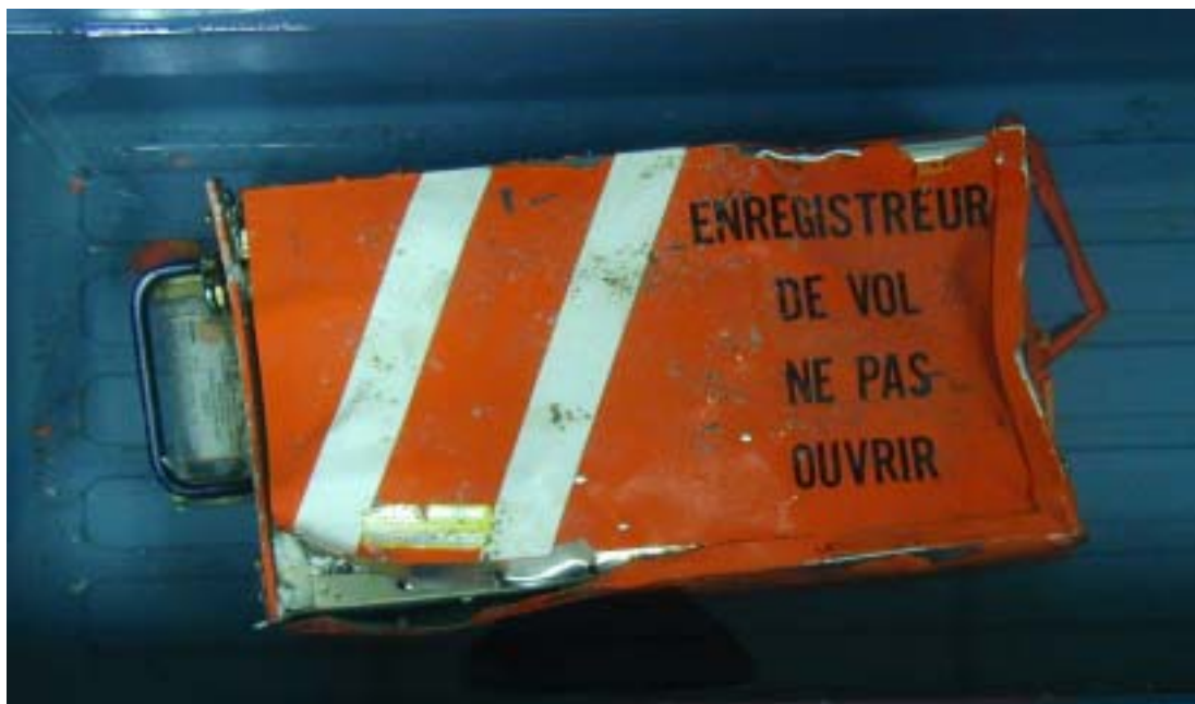
Figure 1.11-1 Damaged CVR in the cooler
