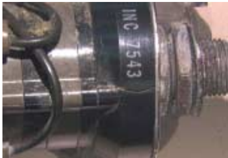
Figure 36: BLEED AIR switch 2.
