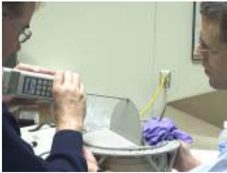
Figure 269: Comparison unit*, door A compression (closing), 1.90 pounds (push at center of door to close door).
