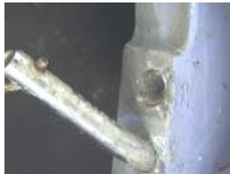
Figure 114: Detail of forward/lower hinge pin bushing in hole.
