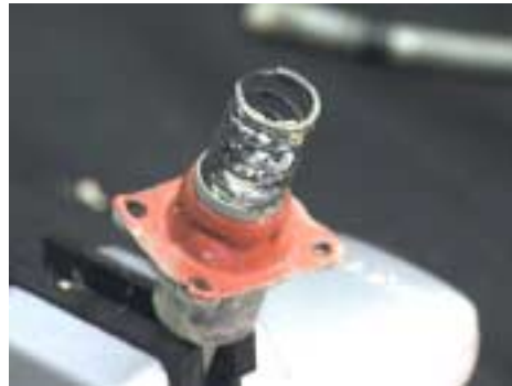
Figure 166 : Diaphragm appears to be intact.
