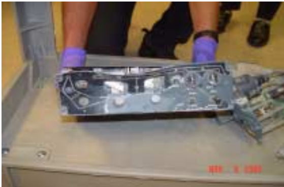
Figure 2 : Flight Engineer's Cabin Pressure Control Selector Panel
