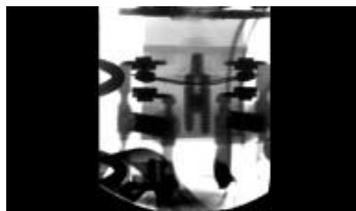
Figure 266 : New switch, open valve, closed contacts.
