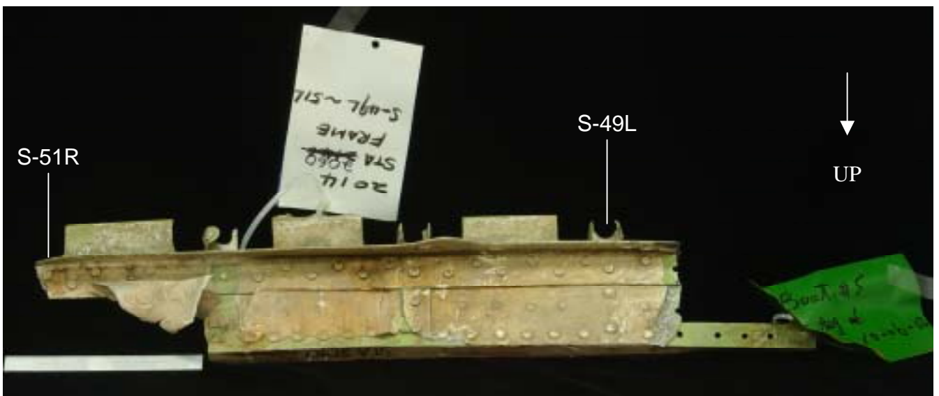
Figure 1.16-114 As received condition of the STA 2060 frame segment. The aft surface is shown in this view.
