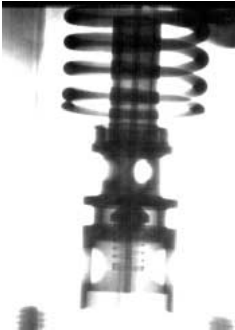
Figure 247: Upper Pressure Relief Valve, control assembly x-ray.
