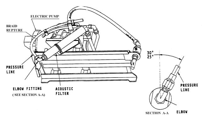
Diagram from the Maintenance Manual showing correct "clocking" of the pressure line when fitting the hydraulic pump to the aircraft.
