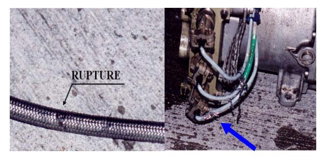
Left photo, showing part of the ruptured flexible pressure hose which chaffed the insulation of phase "C" supply to the electrical hydraulic pump. The arrow at right indicates the resulting damage to this insulation.
