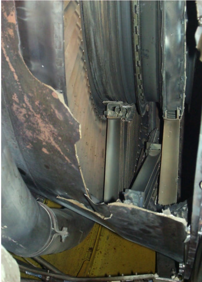
Figure A7. Engine #2 LPT Module, 5 th and 6 th stage (1)
