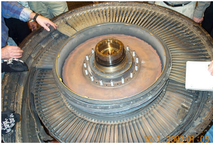
Figure B4. Engine #2 LPT Module - 5 th stage disc revealed
