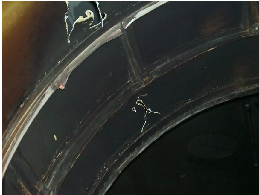
Figure A16. FOD on Engine #1 RH reverse cowl (2)
