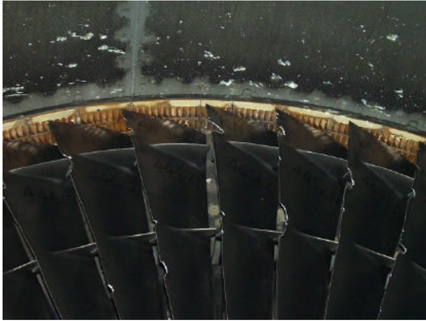
Figure A13. FOD on Engine #1 Fan/Fan Blades (2)
