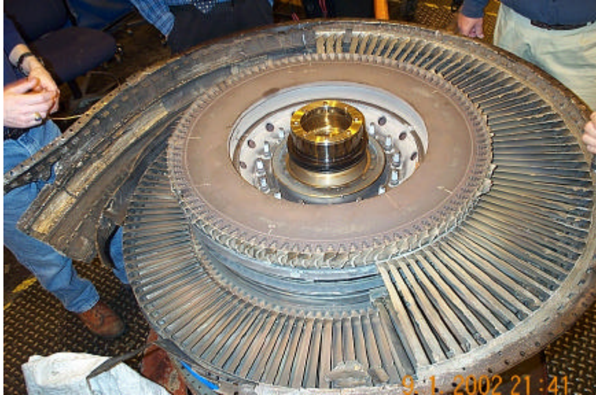
Figure B1. Engine #2 LPT Module (1) - 6 th stage disc on top
