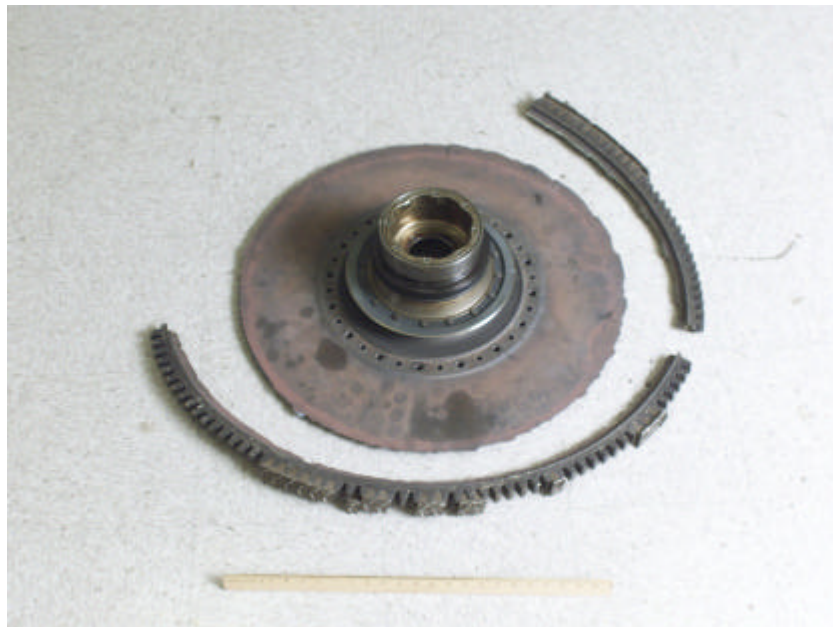
Figure B12. 5 th stage disc - web and two portions of recovered rims
