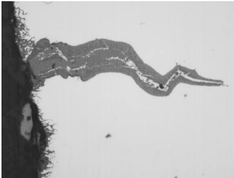
Figure C9. Secondary intergranular crack on forward face (left side)
