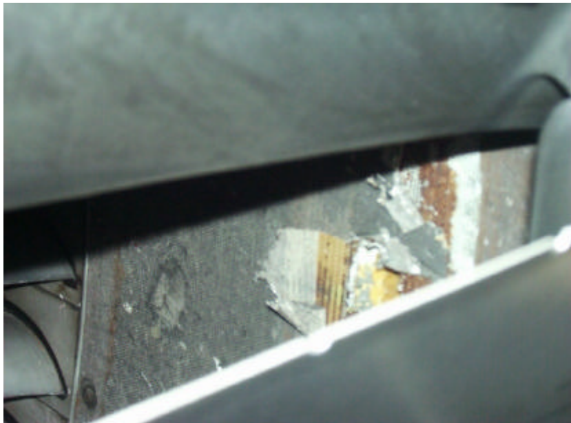
Figure A14. FOD on Engine #1 inner cowling
