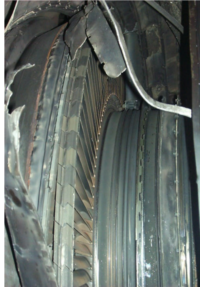
Figure A8. Engine #2 LPT Module, 5 th and 6 th stage (2)
