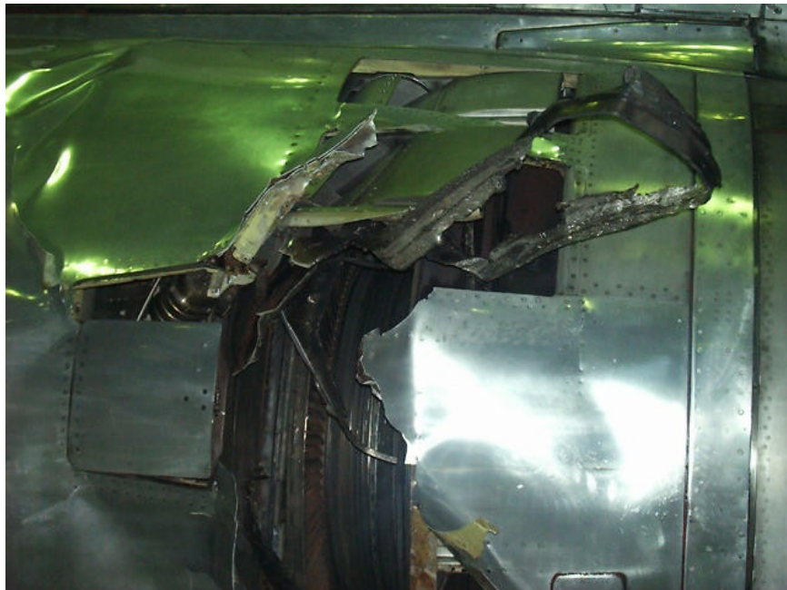
Figure A2. Damage on Engine #2 casing (2)
