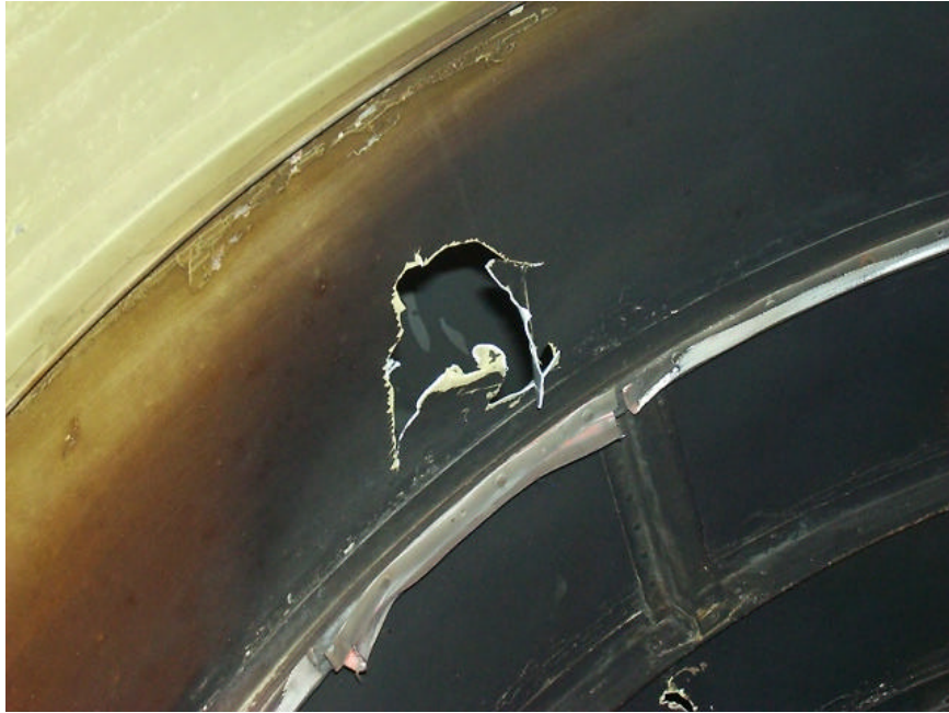
Figure A15. FOD on Engine #1 RH reverse cowl (1)
