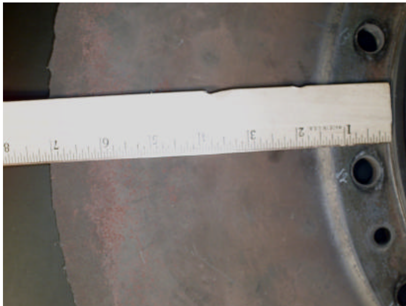
Figure C2. Location of fracture origin on 5 th stage disc web, measured from bore - aft face
