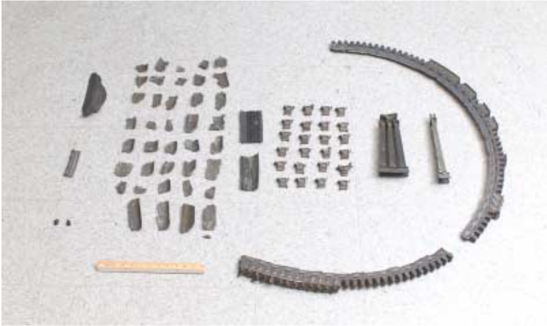
Figure 1. As-received portions of the 5th stage LPT disk showing two pieces of the rim (right side of photograph), and several pieces of vane and blades.
