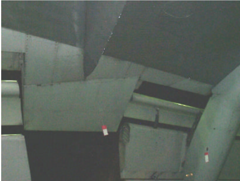
Figure A19. Damage on LH low speed aileron and flap track fairing - tagged debris
