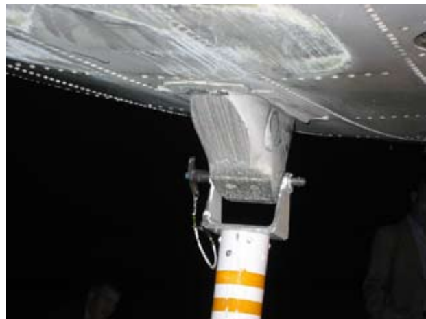
Abrasion damage on fuselage underside
