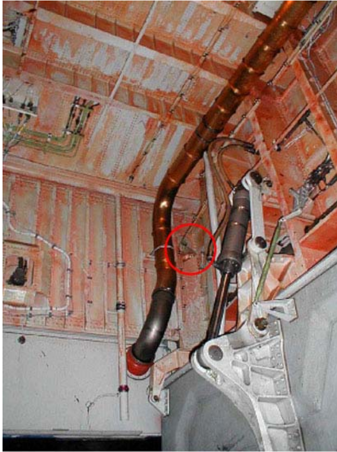
Figure 1 - View inside left main gear bay looking forward at the rear spar of the centre fuel tank. Purge door opening circled in red.
