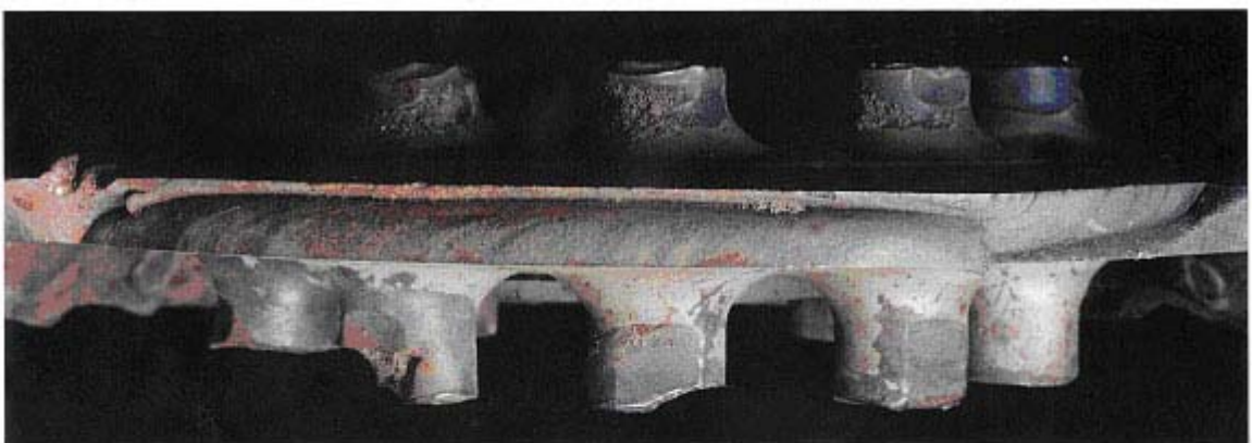
Figure 9 Previous diaphragm failure locations - high pressure turbine
