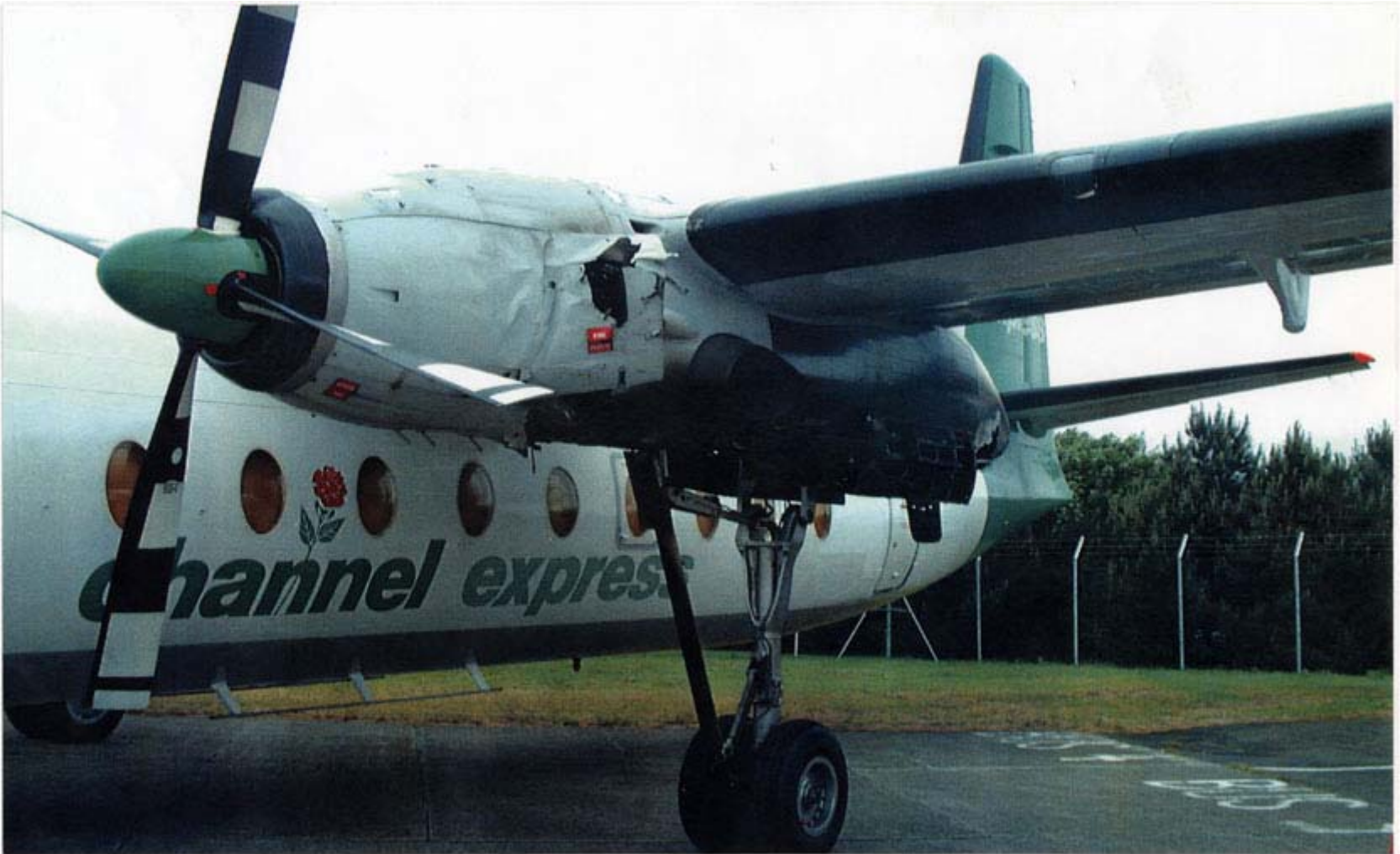
GENERAL VIEW OF LEFT NACELLE SHOWING EXTERNAL DAMAGE
