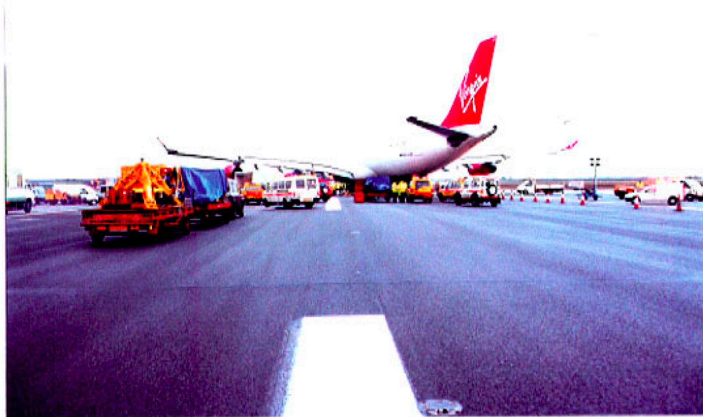
This photograph, taken the following morning, shows the aircraft after jacking and prior to moving. Note the runway centreline markings and aircraft heading. The runway had been repaired by the time this photograph was taken
