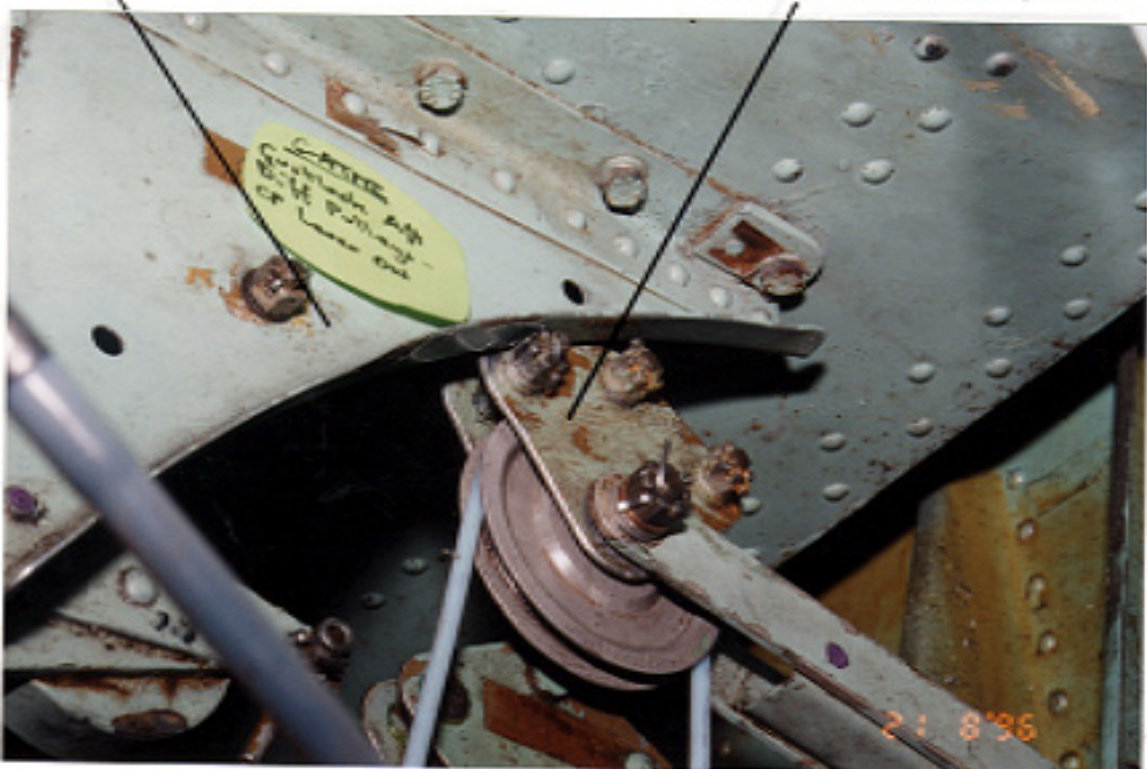
PHOTO 3.2 - AFT DIFFERENTIAL PULLEY FOUL ON BRACKET
