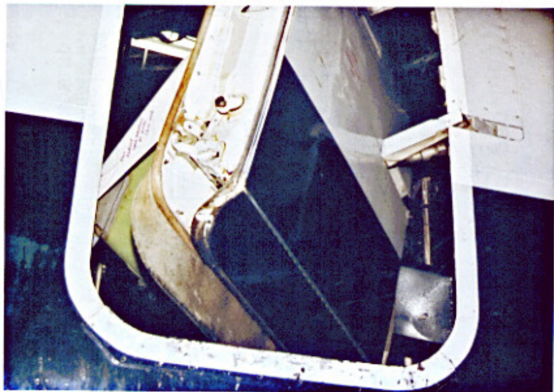
b - Door Position With Witness Marks Aligned-External
