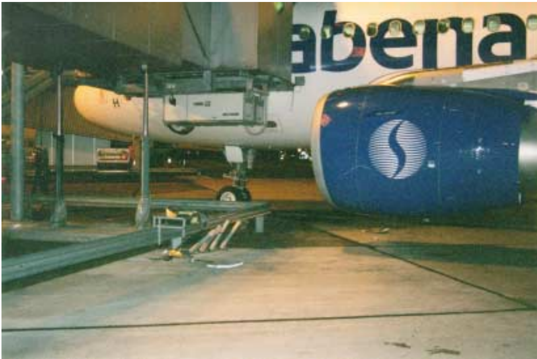
Picture 5. The destroyed stepladder in front of the damaged engine (the stepladder has been removed away from its original position where the damage occurred)
