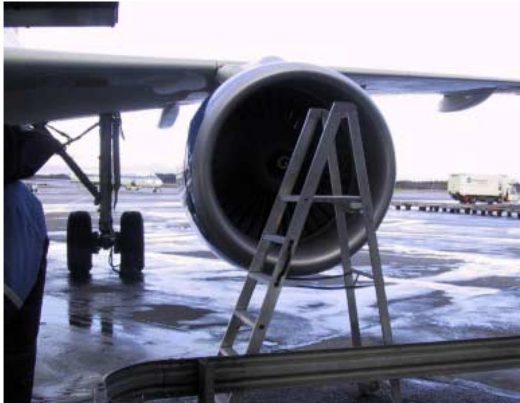
Picture 3. Simulated situation of the position of maintenance stepladder prior to damage
