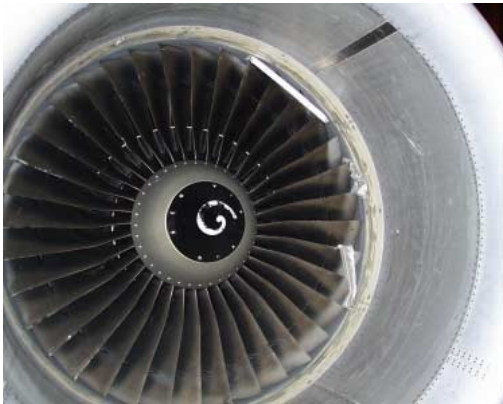
Picture 4. A general photo of the damaged engines air inlet and the parts of the maintenance stepladder in it
