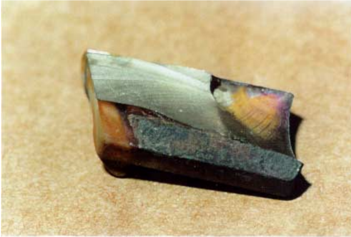
Figure 1. The failed 8th stage compressor rotor blade root
