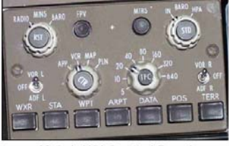
M-Cab HSI Control Panel
