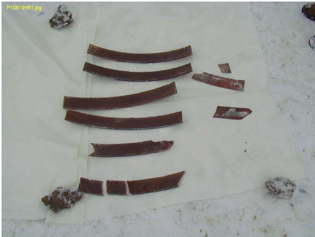
Attachment 12: All loose ice impact panels of the RH engine
