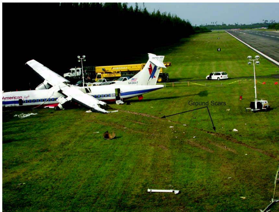
Figure 3. Ground scrape marks and the main wreckage.
