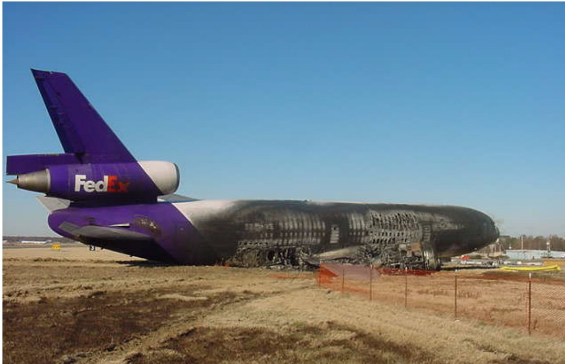
Figure 2. Photograph of the damage to the right side of the airplane.
