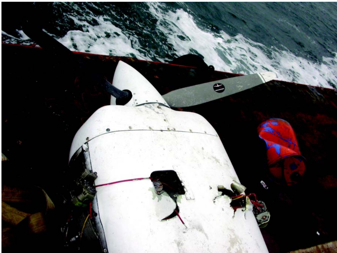
Figure 3. Exterior of the upper outboard engine cowling.
