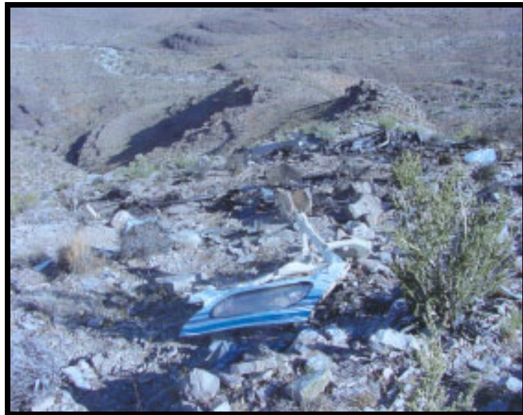
Figure 5. View of crash site showing left door (in foreground) found upslope from IPI.
