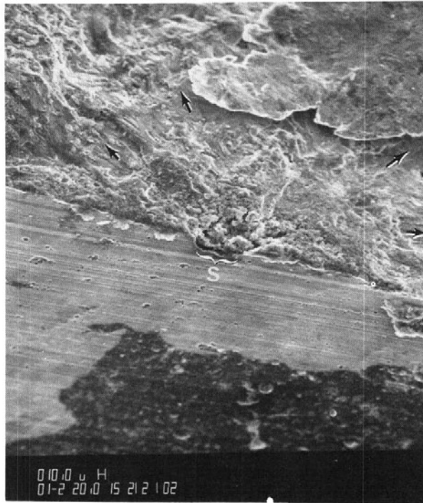
Figure 5. SEM photograph showing secondary origin bracket "S" (see arrow "S" in figure 4 for location). Fracture surface is above origin and hole radius is below. Arrowheads depict fatigue propagation direction. X100
