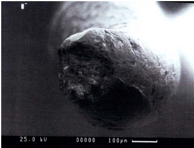
Figure 12. The SEM image shows B fracture surface of the #1 wire. The fracture surface is round and shows clear necking.
