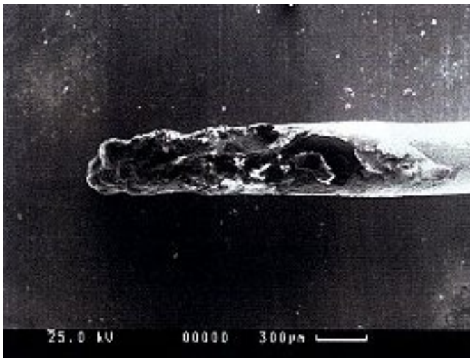
Figure 7. The SEM image shows the P of the positive wire. The lead has necking and the broken surface is a dark brown color, with broken plating and uneven on the substrate.
