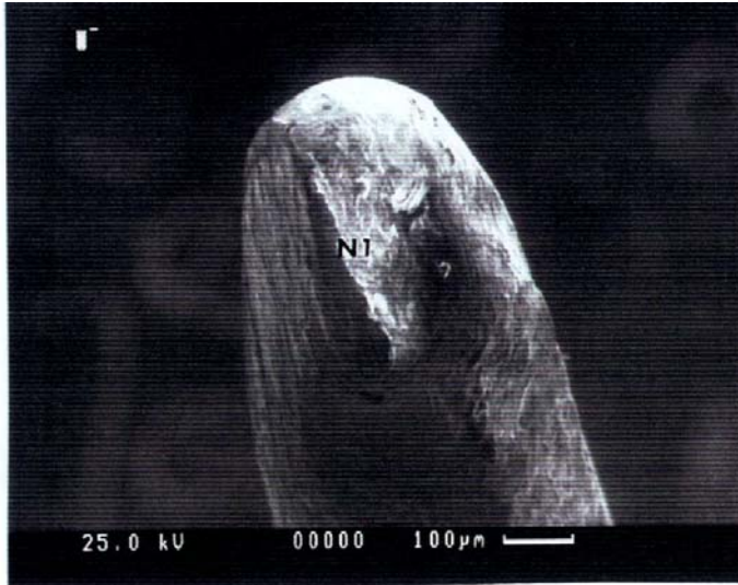
Figure 20. The SEM image shows the N fracture surface of the negative wire. The fracture surface shows it squeezed flat into an almost triangle form.
