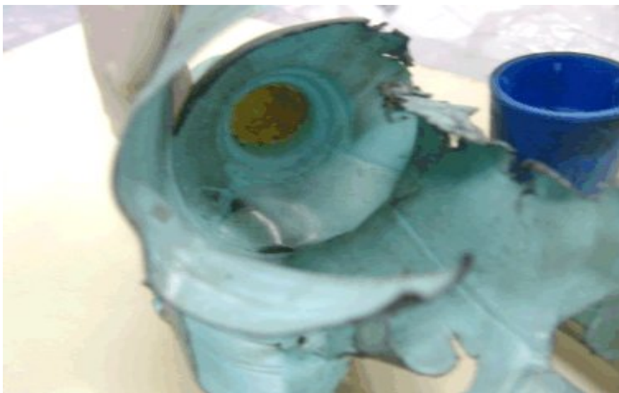
Fig. 1.14-4 A view from the fractured bottle opening, evidence No. 585 showing semi-transparent material.
