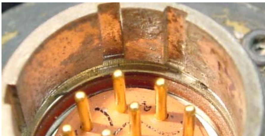
Figure 14. Fluid Tracks and Corrosion in Left Cockpit Gauge
