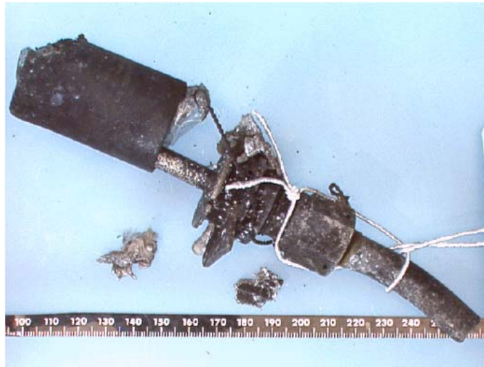
Figure 17. The Condition of the Float Switch
