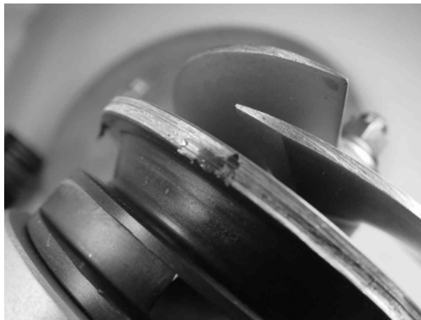
Figure 9. Scoring and Metal Adhered to Outer Diameter of the Impeller of the CWT Left Pump
