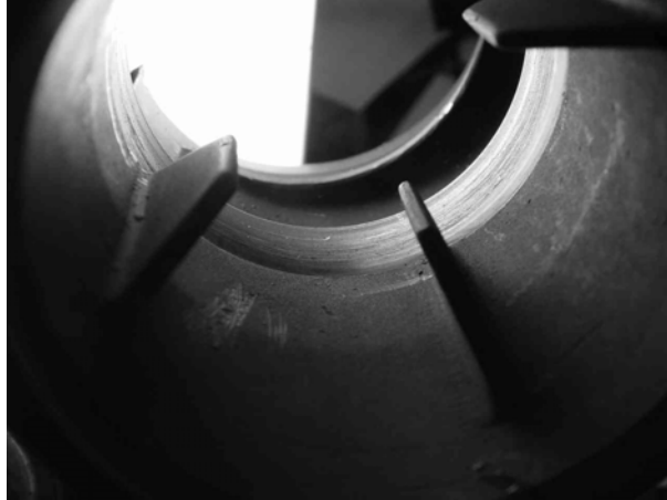
Figure 8. Galling in Aluminum Housing around Inducer and Impeller of the Left CWT Pump
