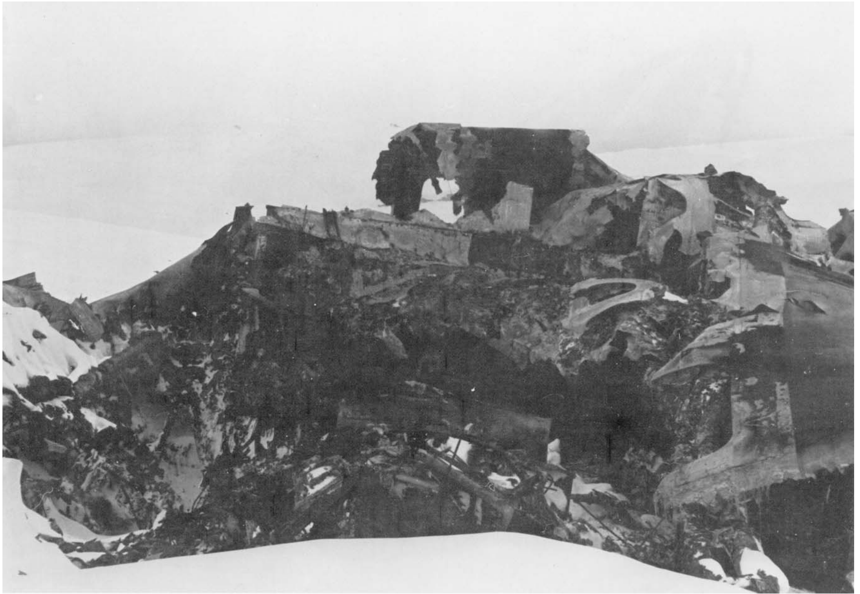
FIG 4 AFTERMATH OF INTENSE FIRE IN CABIN AREA
