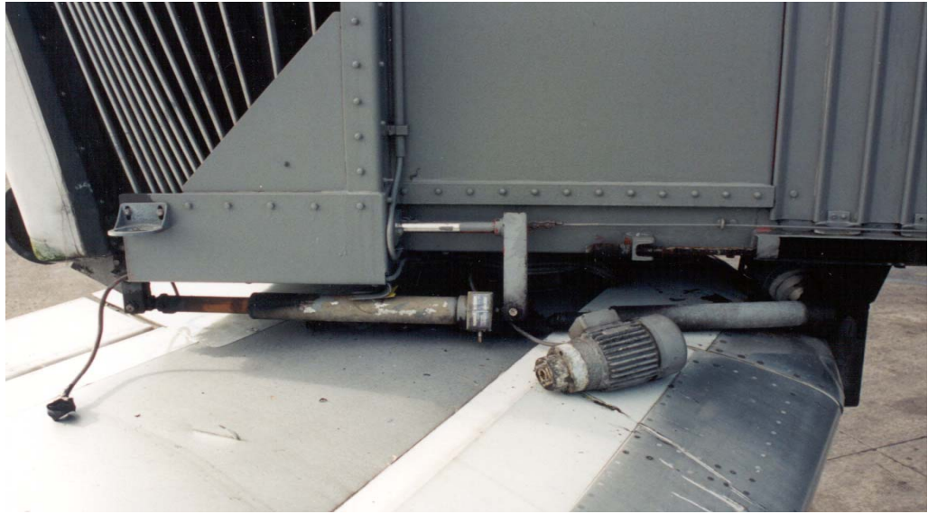
Photo.1 The port wing of EI-CDH following the aircraft's impact with the airbridge on Stand 38.
