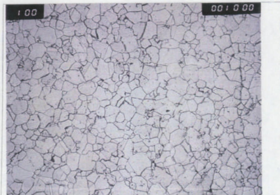
Figure 14. Photomicrograph of section "Y-Y" at the outboard portion of the bore showing typical grain size. Etched with Tucker's reagent. (100X)
