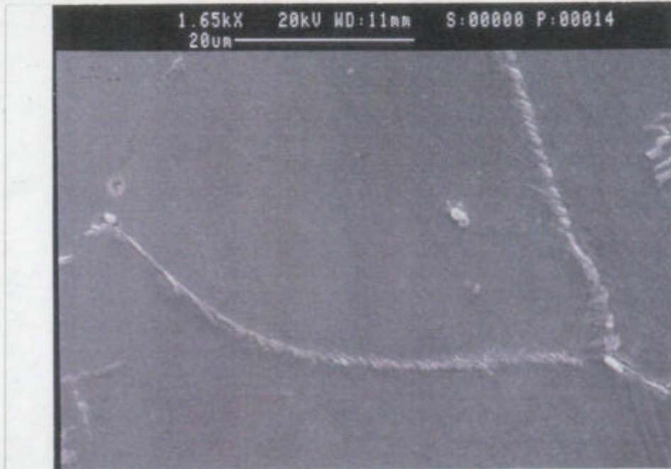
Figure 30. SEM photograph of section "Y-Y" located at the web and below the fracture origin area showing typical microstructure. (1,650X)
