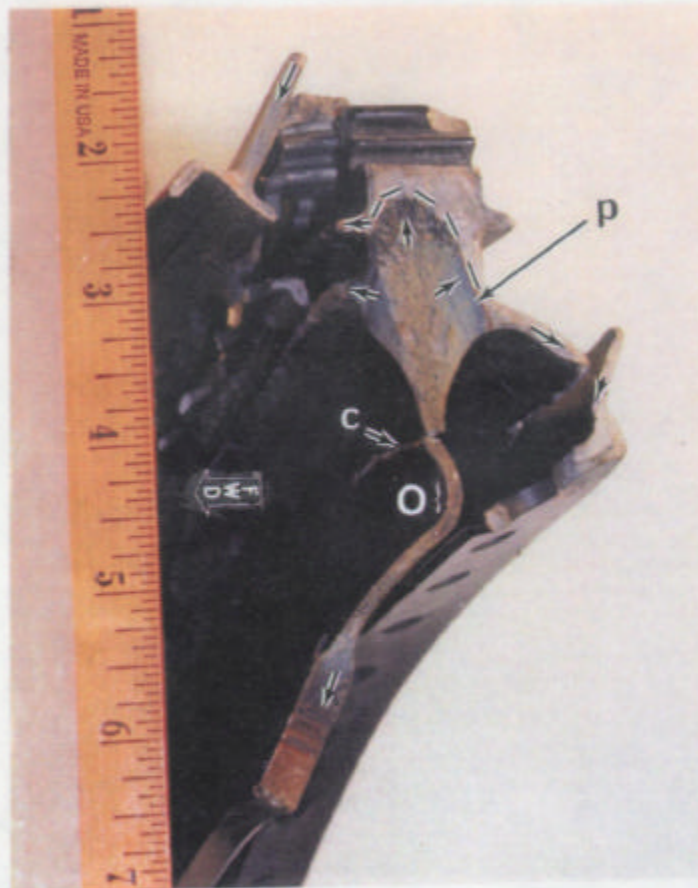
Figure 2. Photograph of fracture "2" on the smaller piece of the disk.
