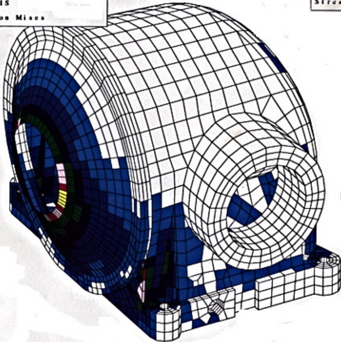
STRESSES DUE TO 100N LOADING IN Y-DIRECTION
