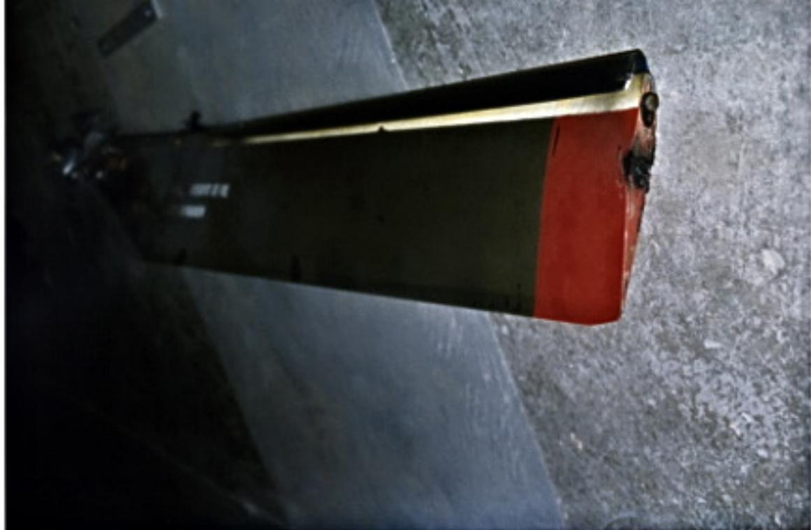
**Figure 6A: Showing TRB s/n 20636 after 198.9kA input to aft tip bolt with minor damage around bolt, but almost complete separation of shield.**
