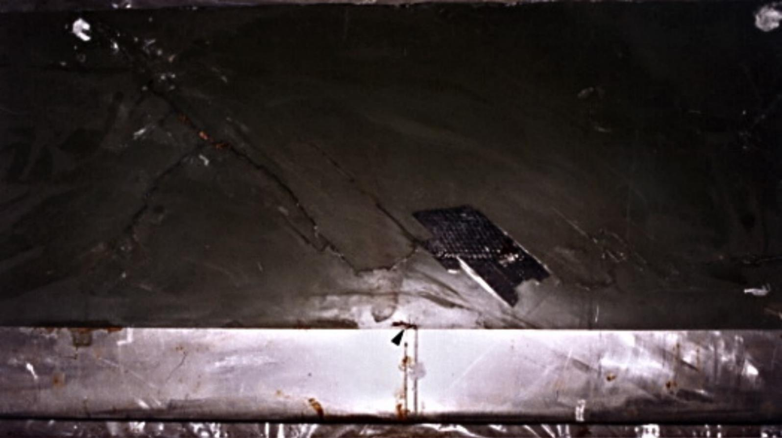
**Figure 9A: Showing localised blade skin damage at overlap of leading edge anti-erosion shield sections due to related arcing on 'Black' MRB.**
