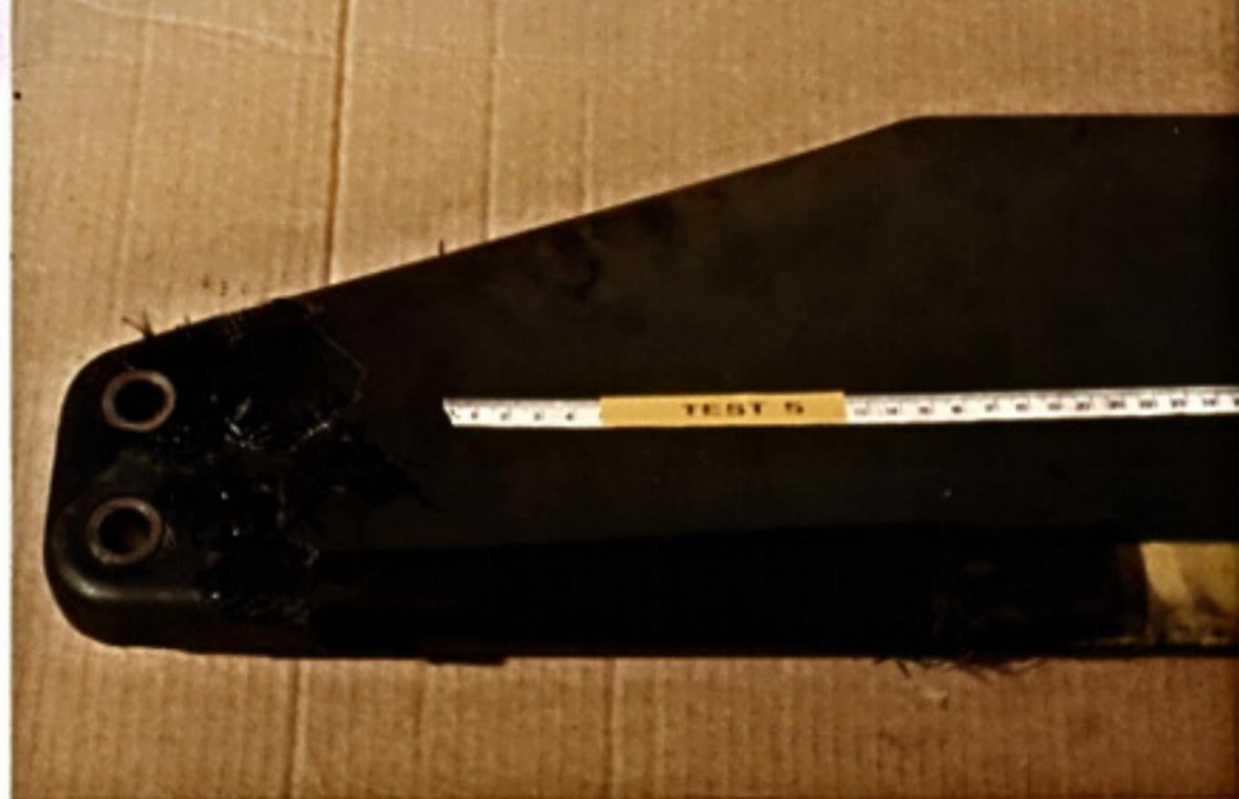
**Figure 10C: Showing marked delamination and disbonding of inboard(left) surface of the root of TRB s/n 20662 after 275.5kA input to aft tip bolt.**
