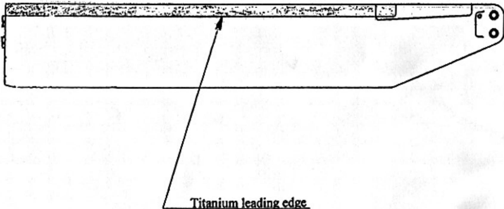
Figure 13A: Showing leading edge anti-erosion shield/conductor design on TRB p/n 332A.12.0020 before modification to improve lightning protection.
