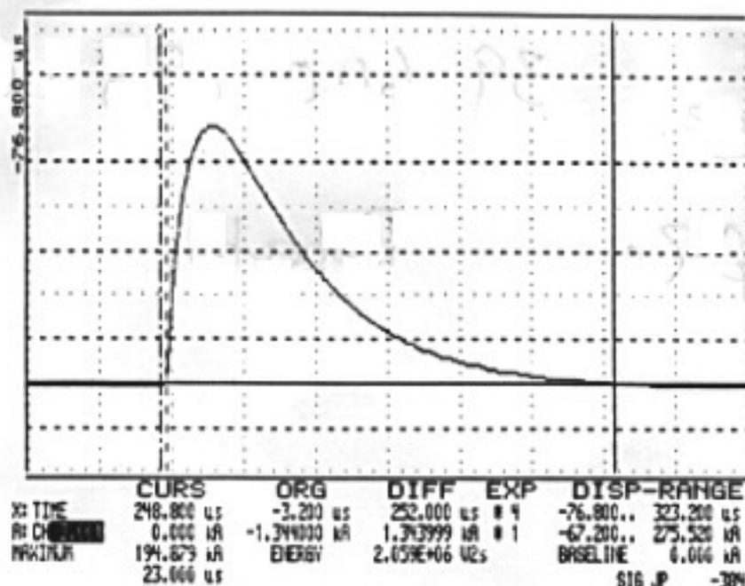
Peak Current is the current amplitude of the positive peak of the waveform.
