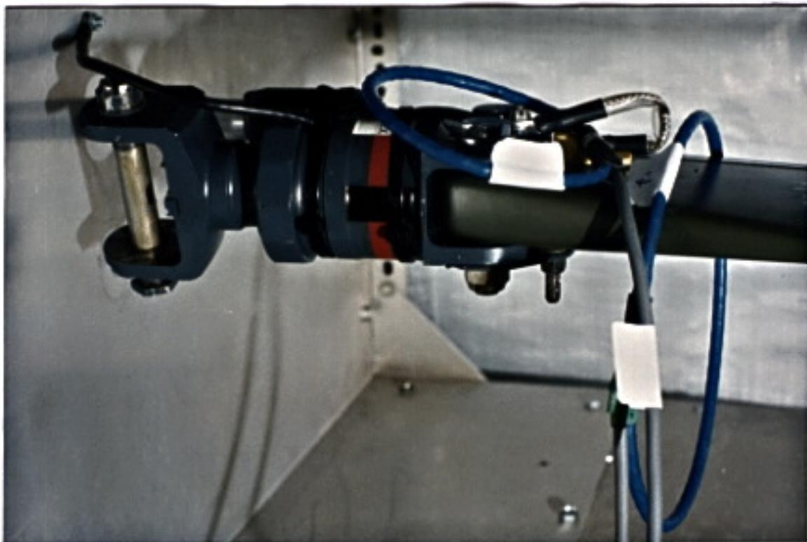
**Figure 1B: Showing first test blade with inboard bonding strap and sleeve bolted to metal end plate, and Rogowski coils in position around root area.**
