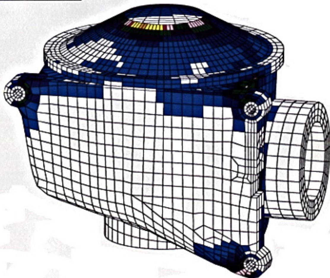
STRESSES DUE TO 100N LOADING IN X-DIRECTION
