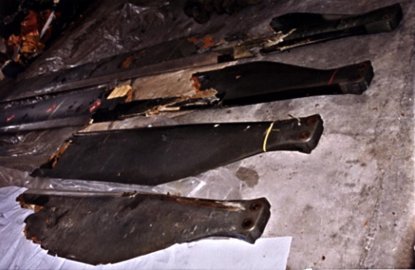
**Figure 9B: Showing all recovered main rotor blade sections, with 'Blue' blade in foreground and 'Black' blade sections in background.**
