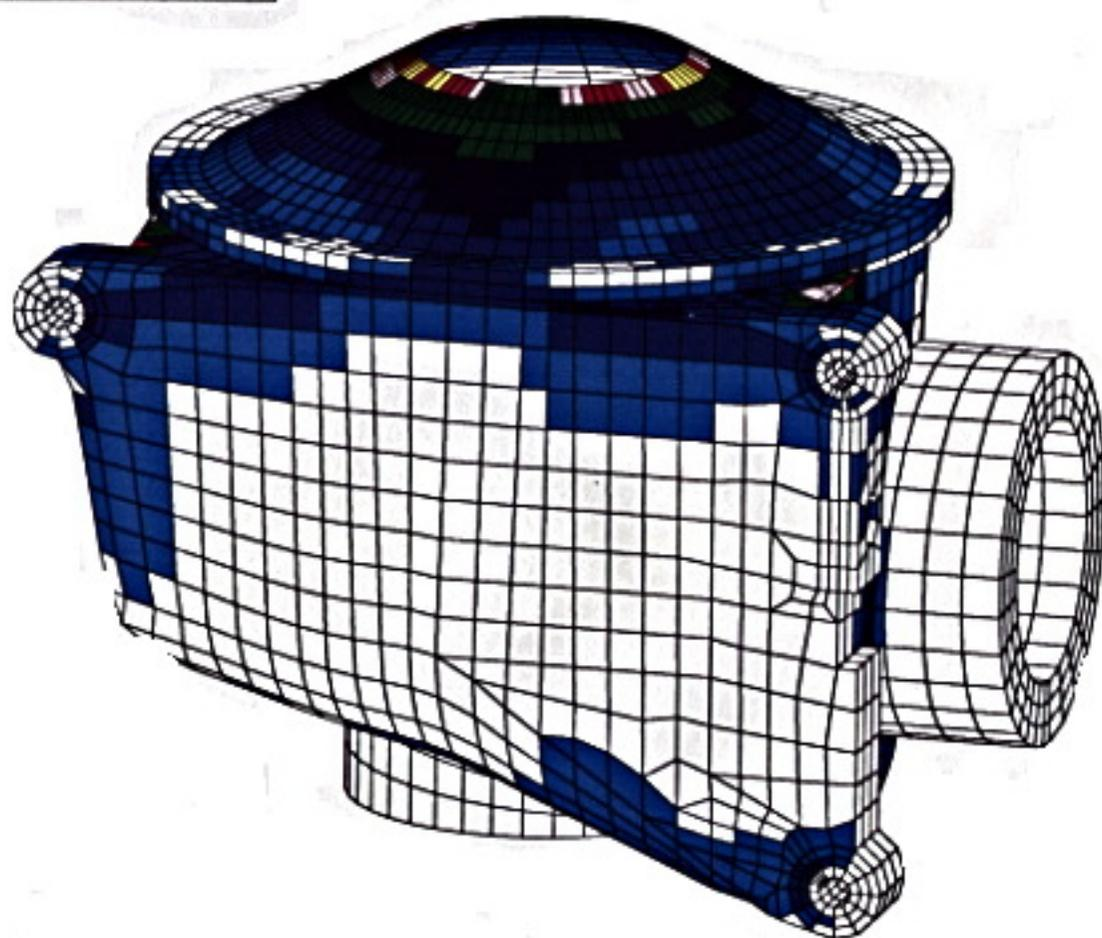
STRESSES DUE TO 100N LOADING IN Y-DIRECTION
