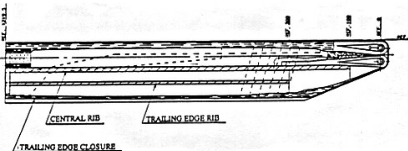
Figure 2: Showing tail rotor blade structure.
