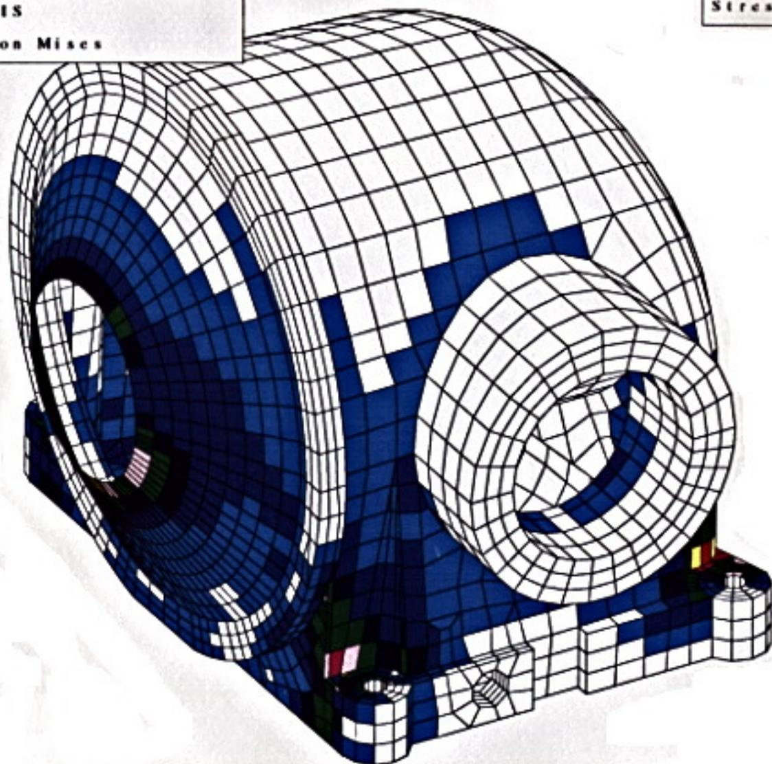
STRESSES DUE TO 100N LOADING IN X-DIRECTION
