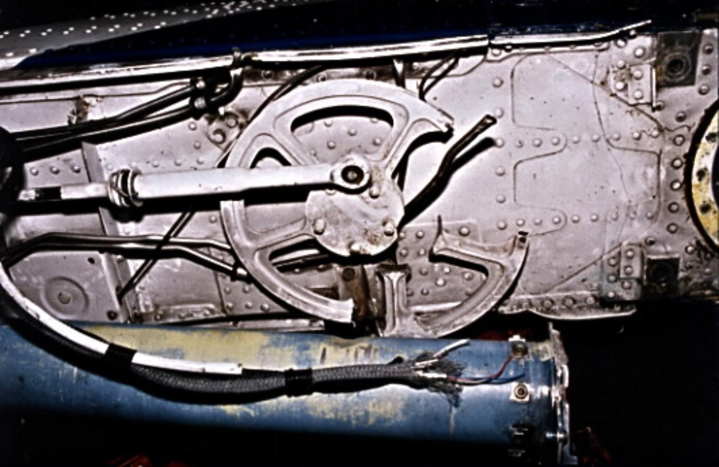
**Figure 7: Showing the four severed hydraulic pipes, with two right side pipes sharply bent around damaged right support flange.**
