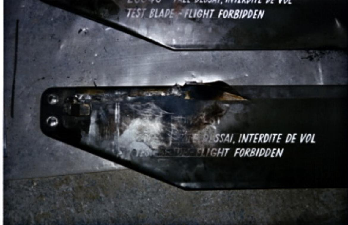
**Figure 9A:** Showing damage to TRB s/n 20732 after 206.9kA input to inboard end of erosion shield, with local peel-back of shield.
