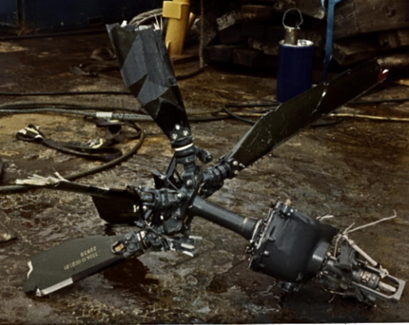
**Figure 4A: Showing recovered tail rotor, gearbox and pitch servo assembly, with 'White' blade root section uppermost.**
