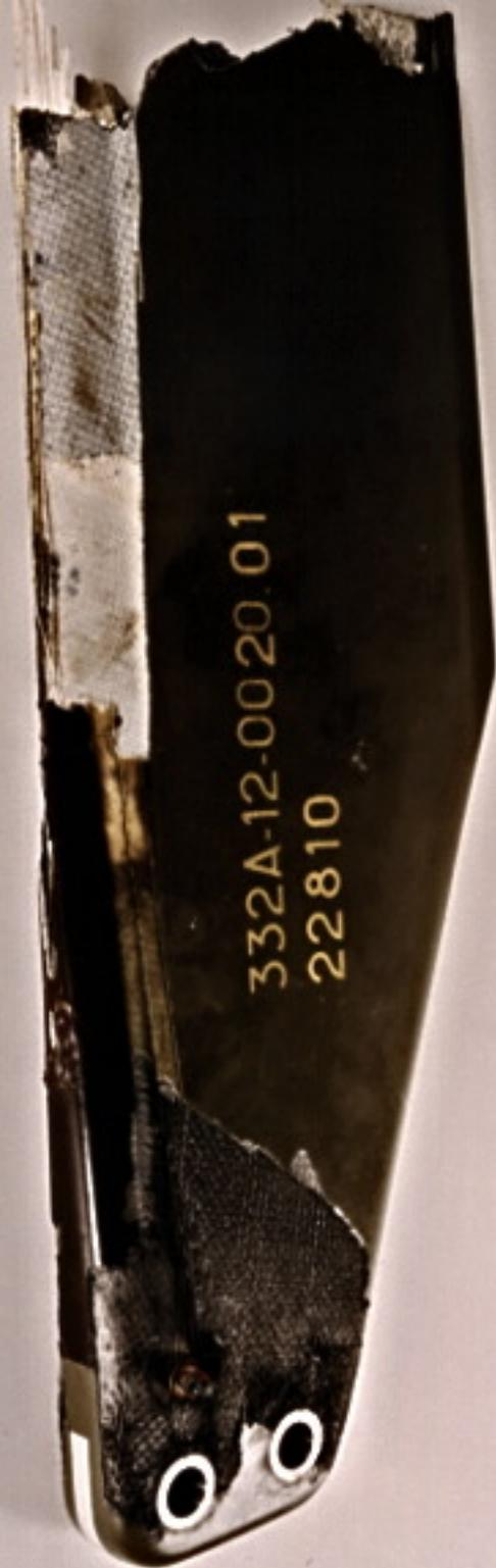
**Figure 10: Showing damaged outboard (right) side of 'White' tail rotor blade, with thermal delamination of root area, full length fissure of composite within bonding strip recess and removal of leading edge skin layer under deatched anti-erosion shield.**
