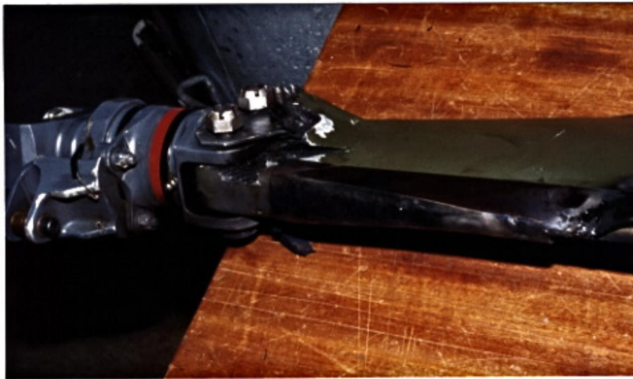
**Figure 11D: Showing very marked carbon fibre disbonding and delamination adjacent attachment bolts on inboard side of above blade.**
