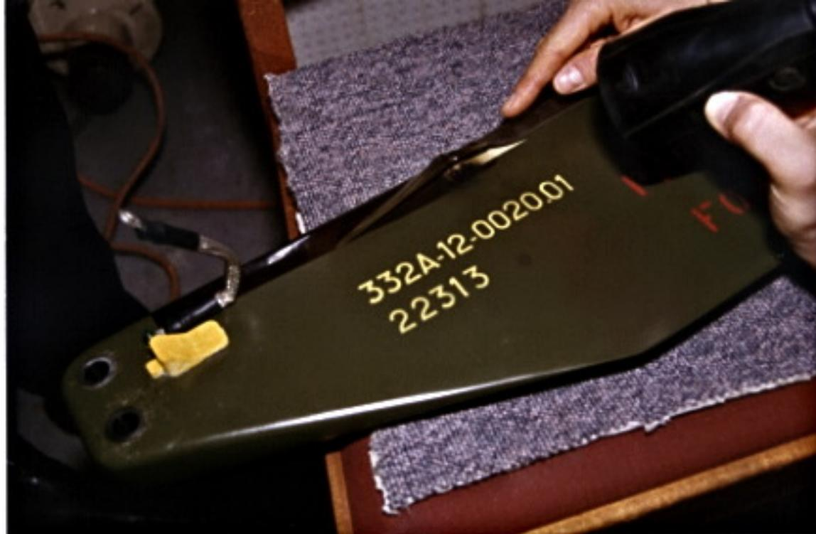
**Figure 2: Showing 'peel-back' of inboard end of anti-erosion shield from brass conducting strip after 12.7kA low energy test (shield tip input).**
