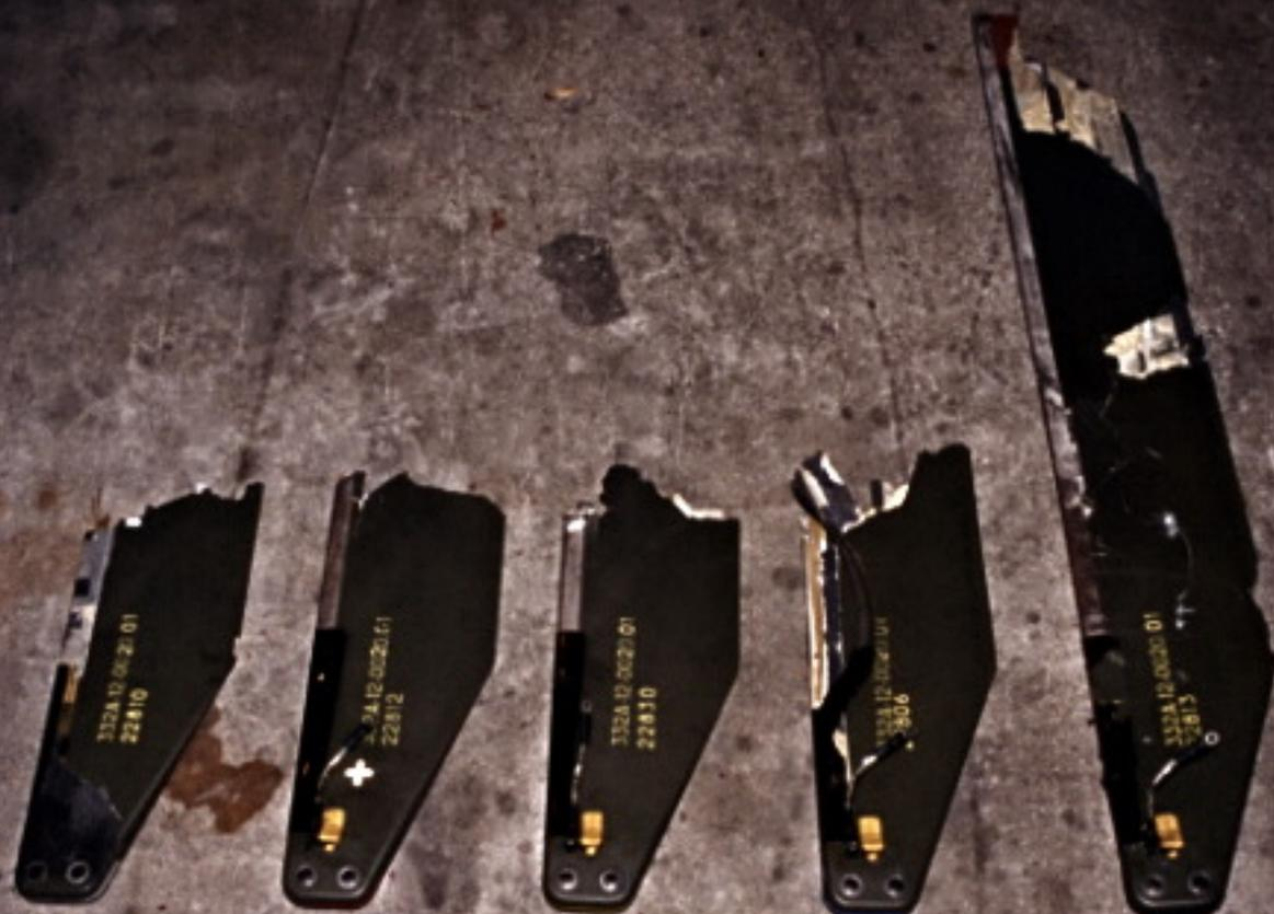
**Figure 13: Showing the recovered tail rotor blade sections with, left to right in this photograph, 'White', 'Red', 'Blue' and 'Black' blades, outboard (right) sides uppermost. Note similar lengths of first four severed blades, caused by rotational penetration into aft side of pylon (Figure 5, A-6).**
