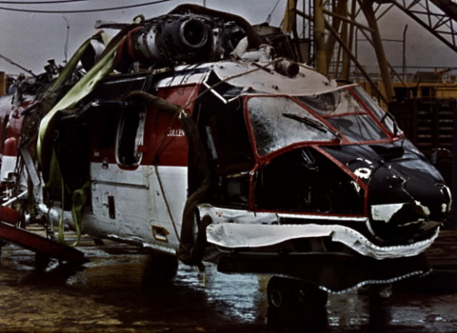
**Figure 14: Showing the recovered helicopter onboard MSV Stadive without its main rotor head and main gearbox assembly which detached during the first associated 'lift' from the seabed and was recovered before the main airframe structure shown here.**
