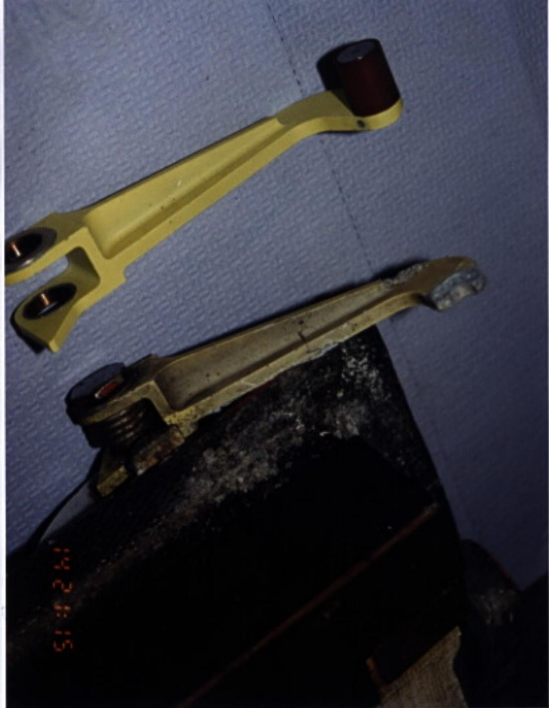
Figure 5: Showing hook-shaped broken end of spring-loaded arm at upper forward corner of left main door, after detachment of roller end, with new arm/roller for comparison; aft arm on this door and forward arm on right door were also broken in this manner.
