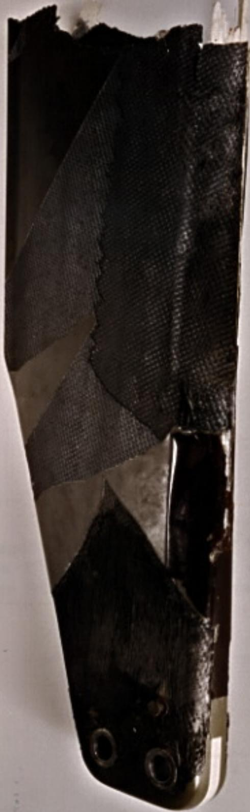
**Figure 11: Showing damaged inboard (left) side of 'White' tail rotor blade, with thermal delamination of root area and general delamination outboard, including the leading edge from which the anti-erosion shield detached.**
