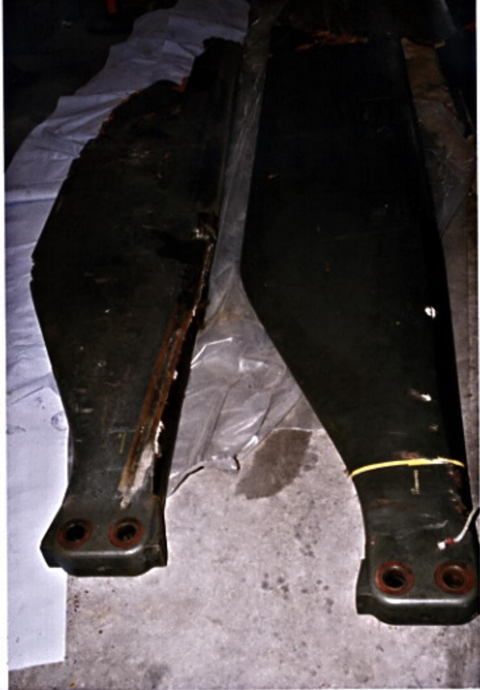
**Figure 8: Showing recovered inboard section of 'Blue' main rotor blade with bonding strip missing, alongside 'Yellow' MRB for comparison.**
