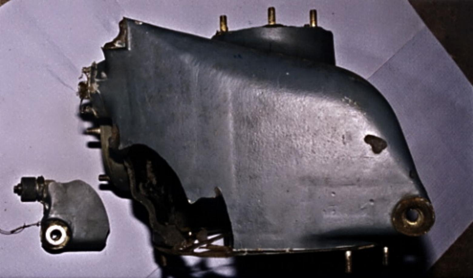
**Figure 6: Showing failed lower attachments of gearbox (left attachment is upper one in this photograph, right is lower).**
