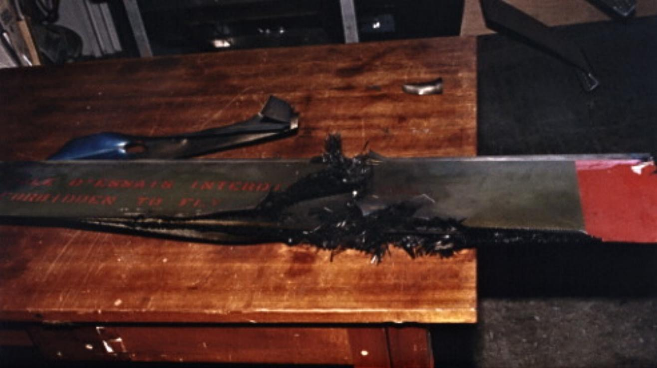
**Figure 11A: Showing gross damage to aerofoil of TRB s/n 22313 after 253.3kA input to trailing edge, 34cm from tip.**
