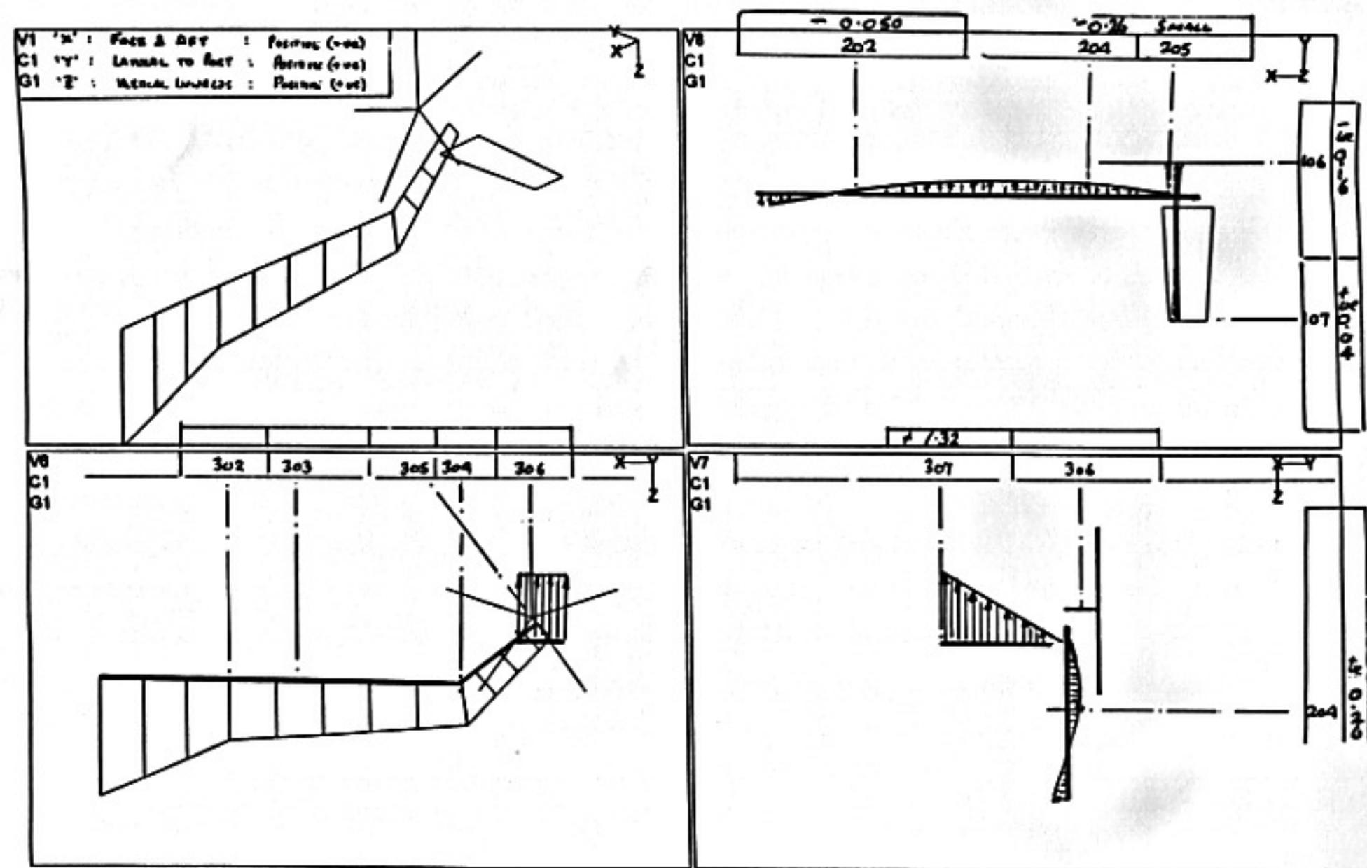
Figure 4: Showing measured overtone lateral bending/tail roll mode at 22.35Hz
