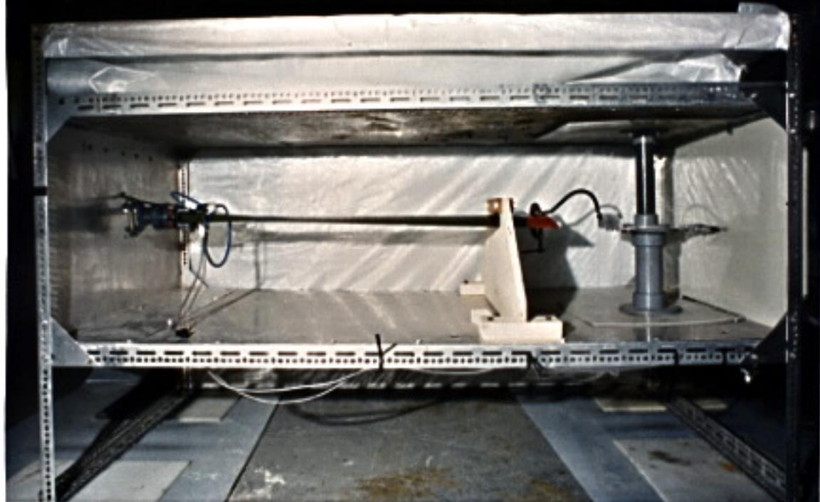
**Figure 1A: Showing LTT test cell used for simulated lightning strikes on sample tail rotor blades, as described earlier in Enclosure 2, section 8.1.**
