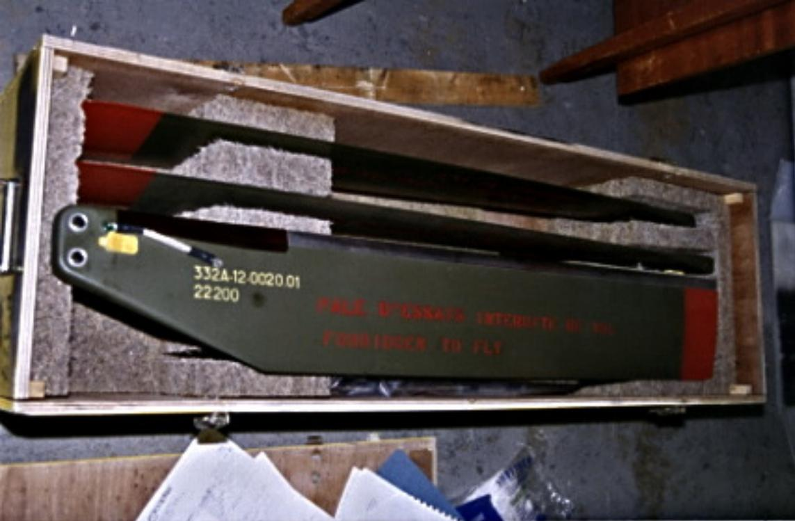
**Figure 3: Showing a sample tail rotor blade with leading edge anti-erosion shield, plastic cover overlying brass strip and braided bonding strap to root bolt.**
