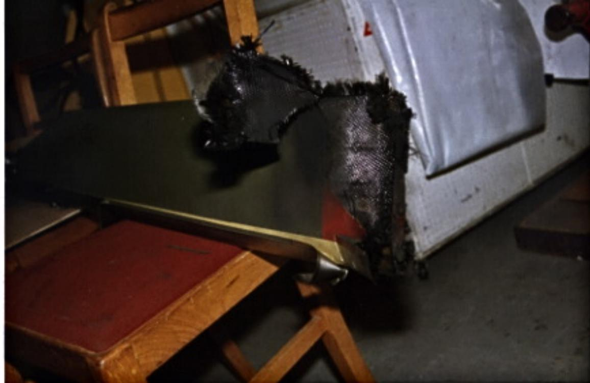
**Figure 4: Showing tip damage to TRB s/n 20667 after 180.1kA input to trailing edge tip, with peel-back and general debonding of erosion shield.**
