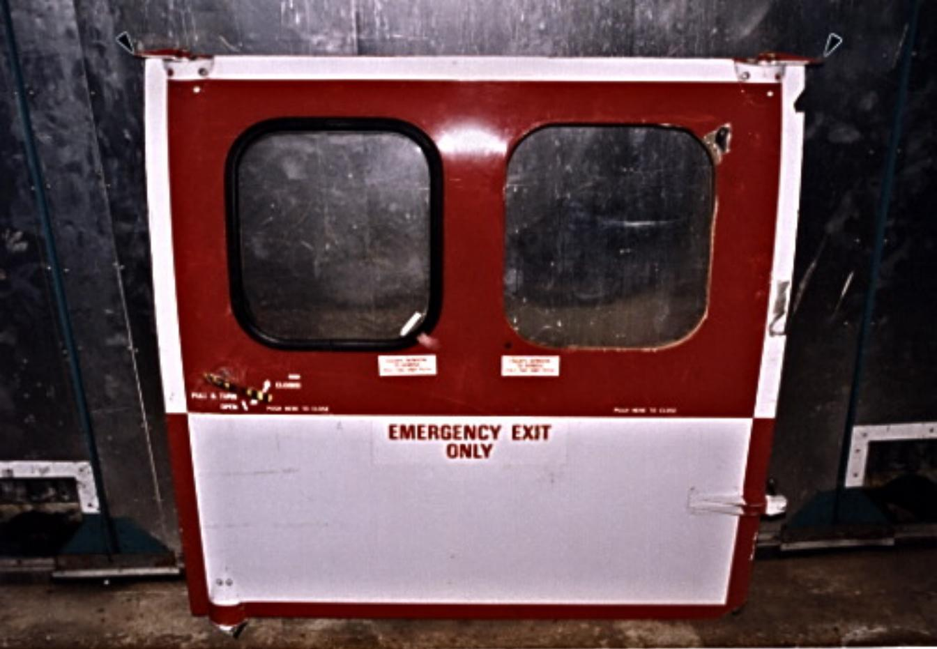
**Figure 2: Showing right main door emergency exit with both spring-loaded arms arrowed.**
