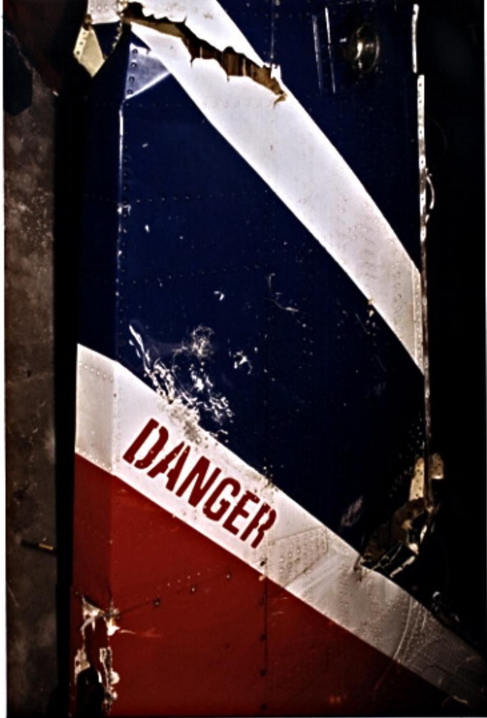
**Figure 5: Showing deep gash in trailing edge of tail boom pylon and tail rotor blade impact damage on right side.**
