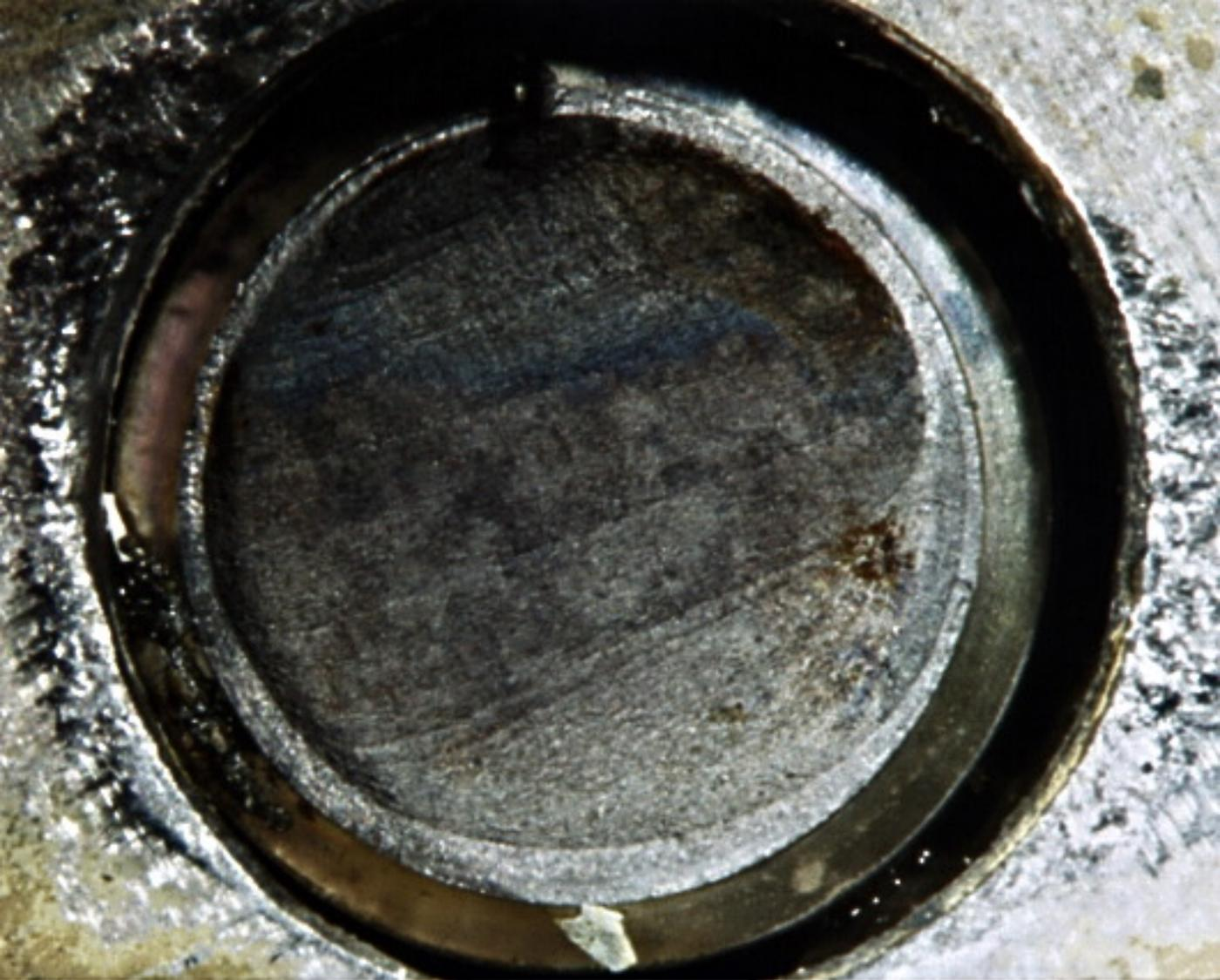
**Figure 12B: Showing fracture surface of lower (threaded) end of tail rotor gearbox upper attachment bolt, with shallow (bright) annular band of initial radial fatigue propagation from the thread root, and secondary bending fatigue striations clearly evident emanating from upper arc, before the final overload failure evident within lower segment of fracture.**
