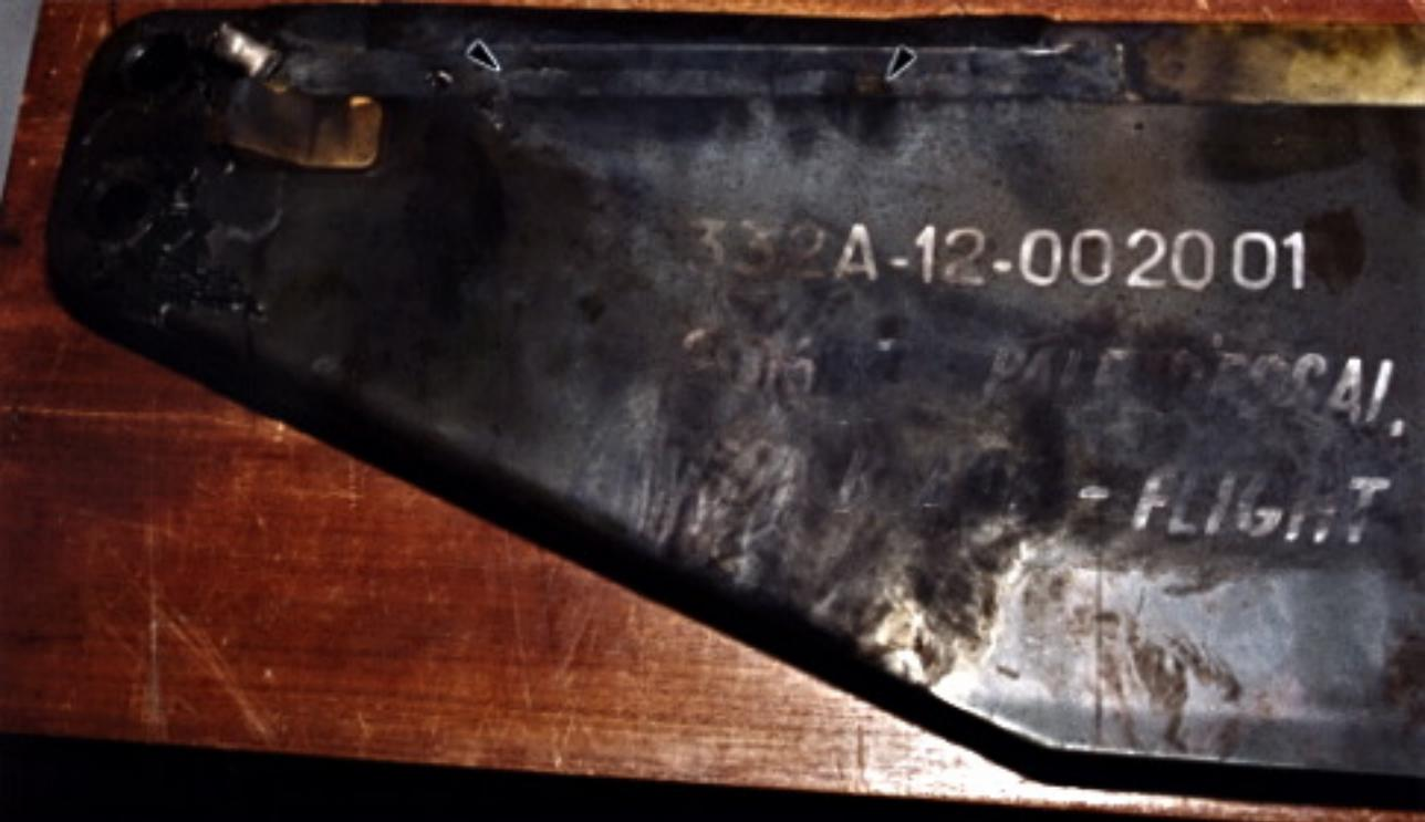
**Figure 12C: Showing almost full length 'fissure'(between arrows) within substrate uncovered by loss of brass conducting strip, and root damage adjacent attachment bolt bushes on TRB s/n 20697.**
