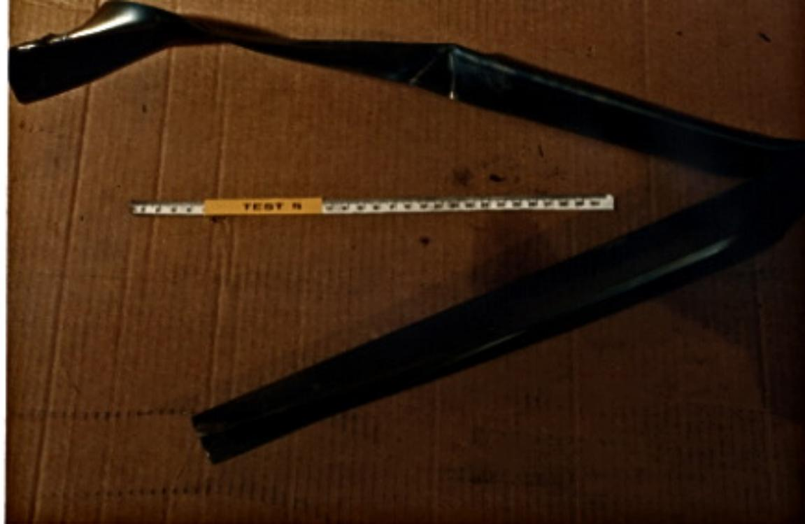
**Figure 10A:** Showing detached and badly deformed erosion shield after 275.5kA input to aft tip bolt on TRB s/n 20662.
