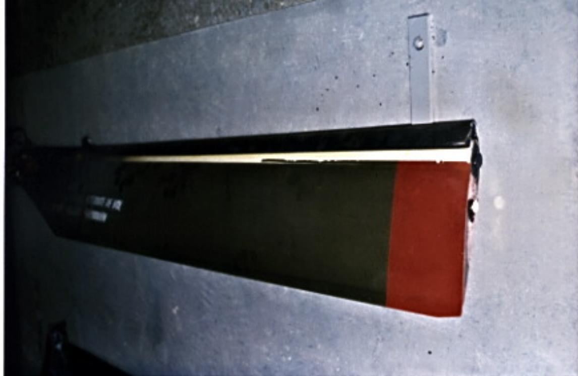
**Figure 7A:** Showing TRB s/n 20625 after 194.9kA input to forward tip bolt with minor damage around bolt and to erosion shield tip, but almost complete separation of shield.
