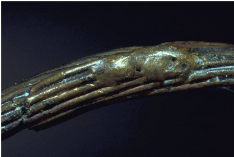
Exhibit 1-3029, from 10 AWG Left Emergency AC Bus Feed (magnification X10)
