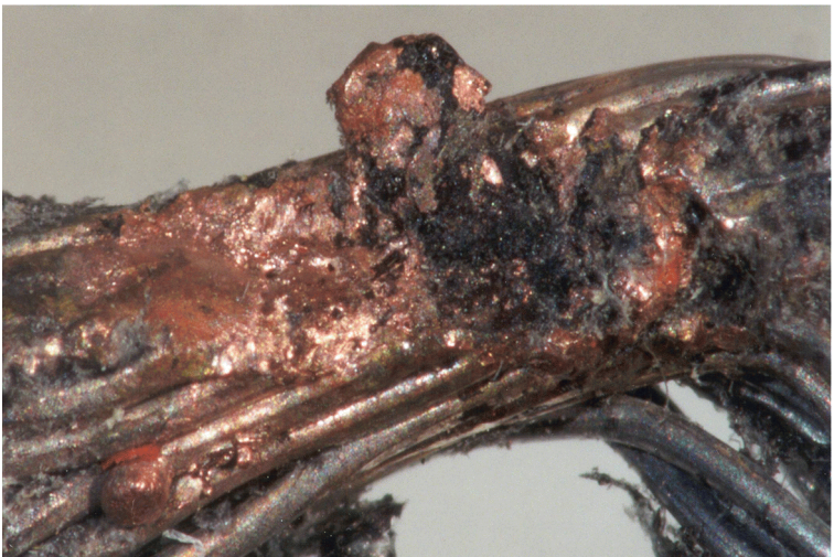
Exhibit 1-14723, from 12 AWG IFEN Power Cable (magnification X22)
