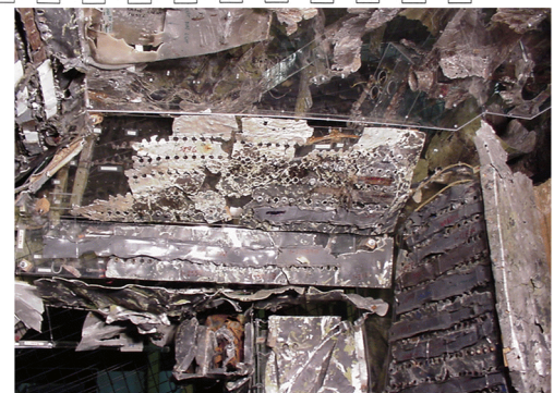
Right Side Cockpit in Reconstruction Mock-Up Showing Upper and Lower Avionics CB Panels
